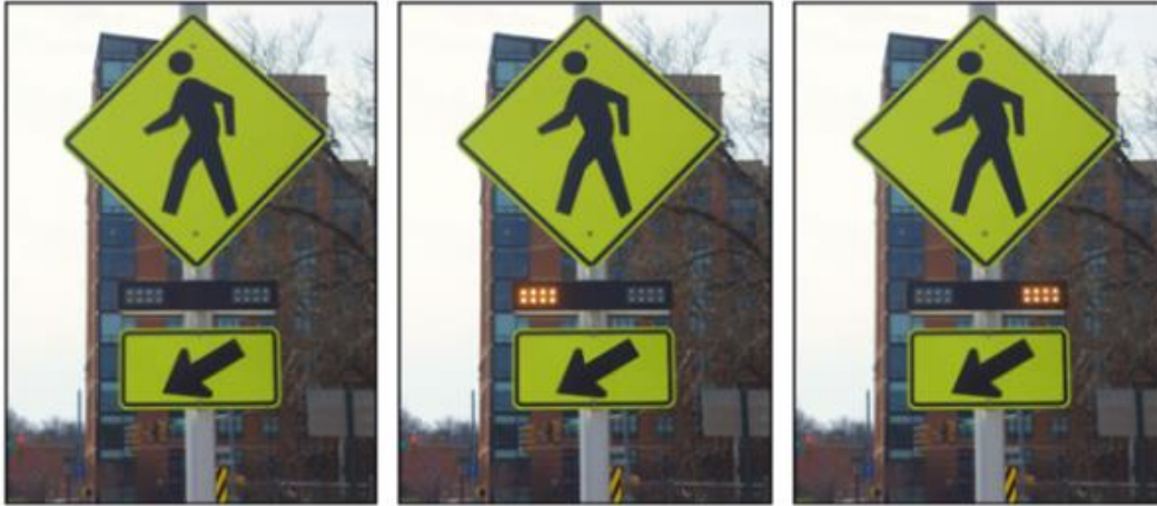
Figure 2.3 Pedestrian-Actuated Rectangular Rapid-Flashing Beacon
