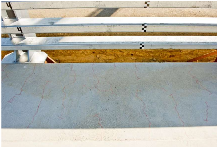
Figure 3-1. Point of Impact 66 inches (1.7 m) Upstream of Post 4
