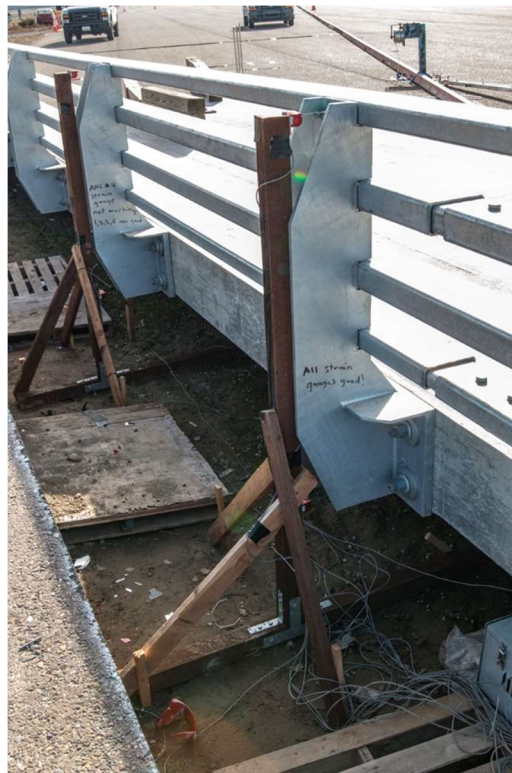
Figure 3-23. Posts 3 and 4 String Pot Mount Supports
