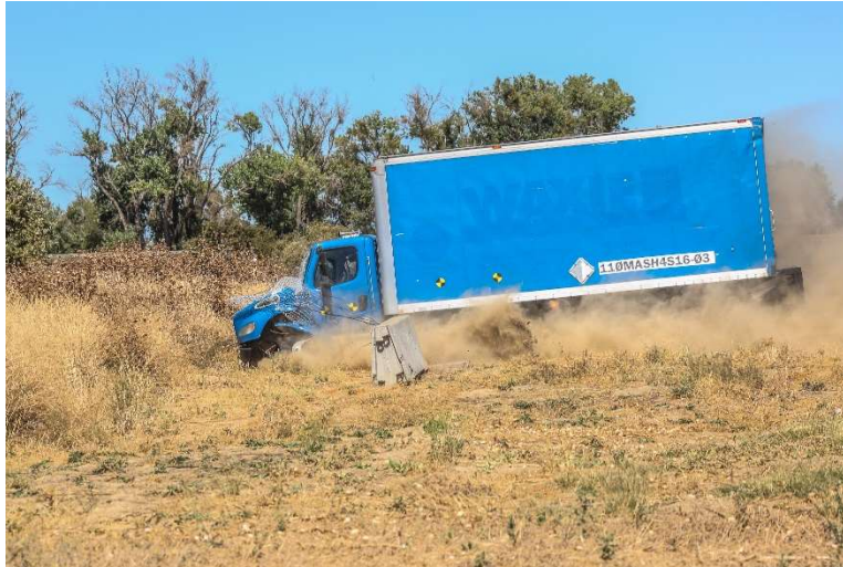
Figure 3-40. 110MASH4S16-03 Impact with Fence
