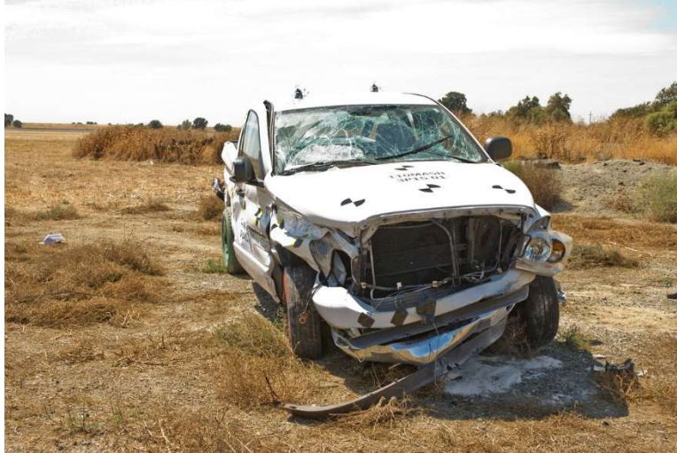
Figure 3-11. 110MASH3P15-01 Dodge Ram 1500 Damage (Front)
