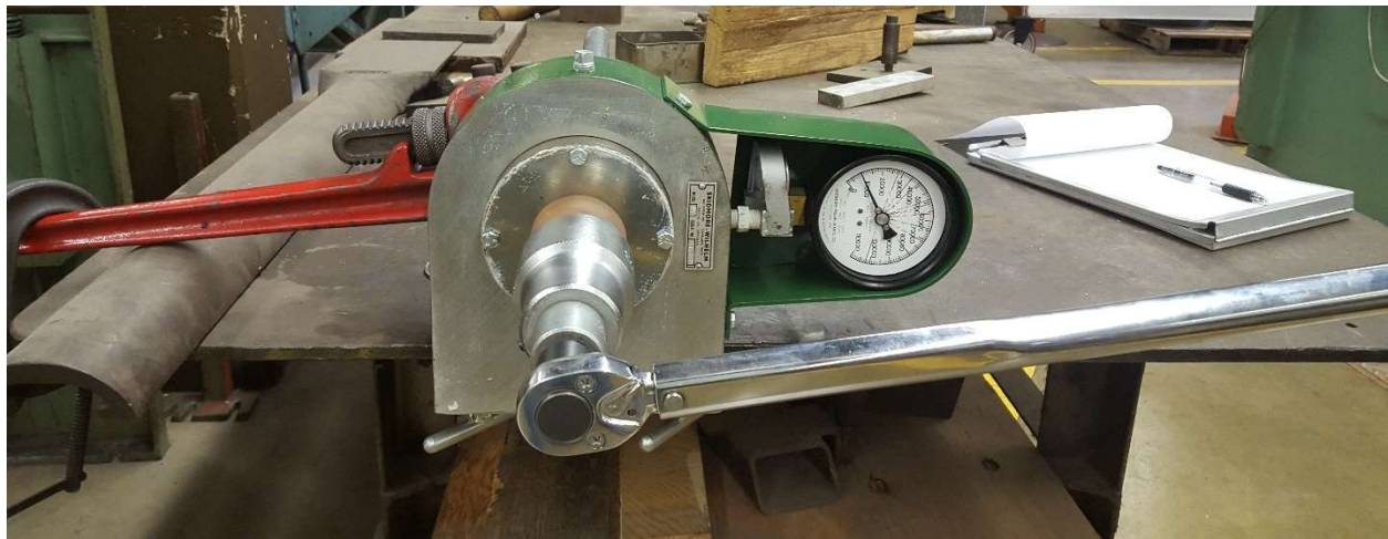
Figure 8-42. Skidmore-Wilhelm Bolt Tension Machine
