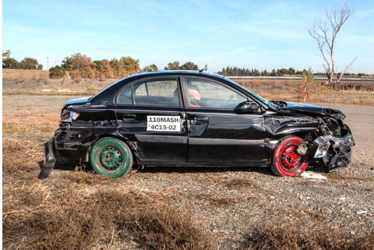
Figure 3-25. 110MASH4C15-02 Kia Rio Damage (Side)
