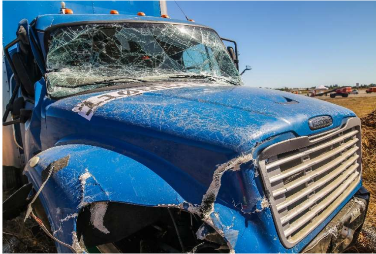
Figure 3-47. 110MASH4S16-03 Front End with Fence Removed
