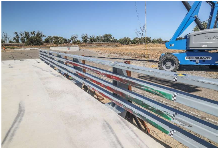
Figure 3-36. 110MASH4S16-03 Green (Front Tire) / Red (Rear Tire)
