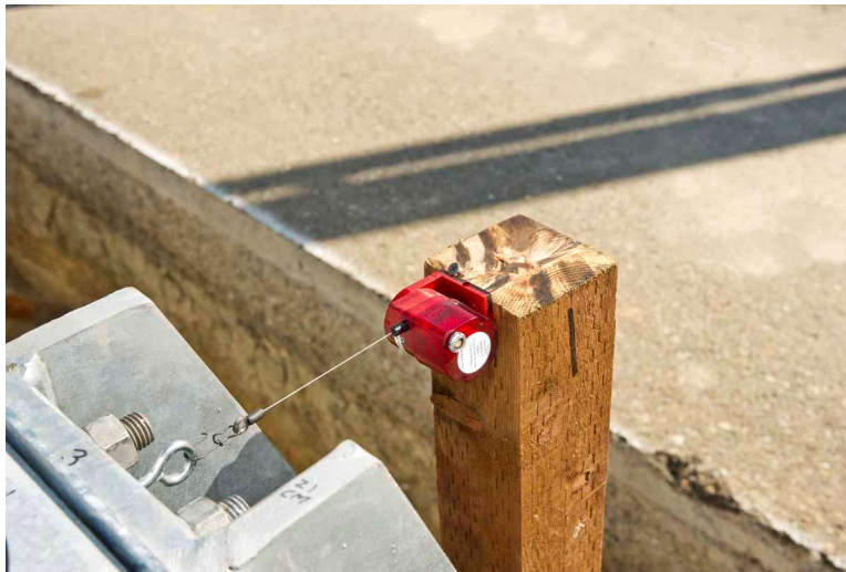
Figure 3-8. String Pot Installed on Upper Post
