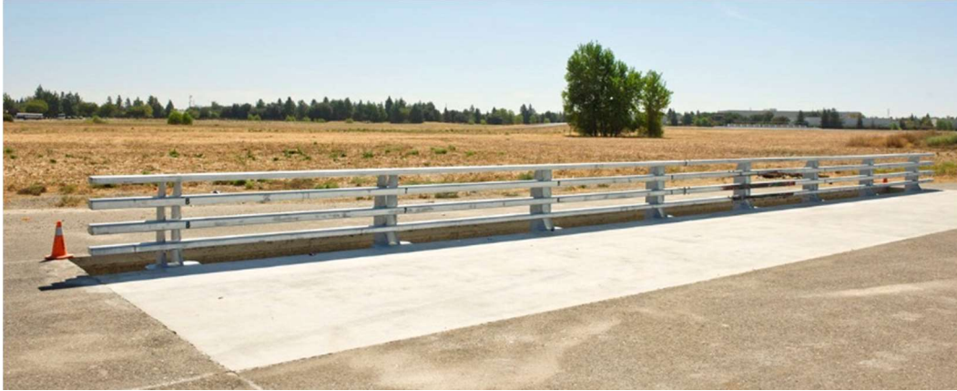
Figure 3-5. CA ST-70SM Side Mounted Bridge Rail after 2270P Vehicle Impact
