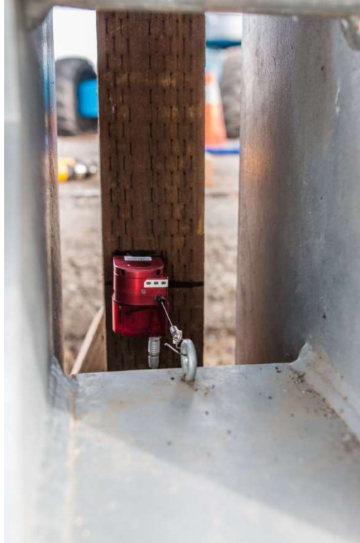
Figure 3-24. String Pot Installed on Base of Post
