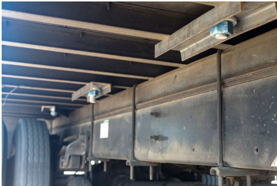
Figure 8-32. 110MASH4S16-03 Vehicle Ballast Mounted in with C-Channels Sections
