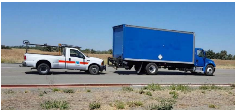
Figure 8-30. 110MASH4S16-03 F350 Push Vehicle and the 10000S Test Vehicle
