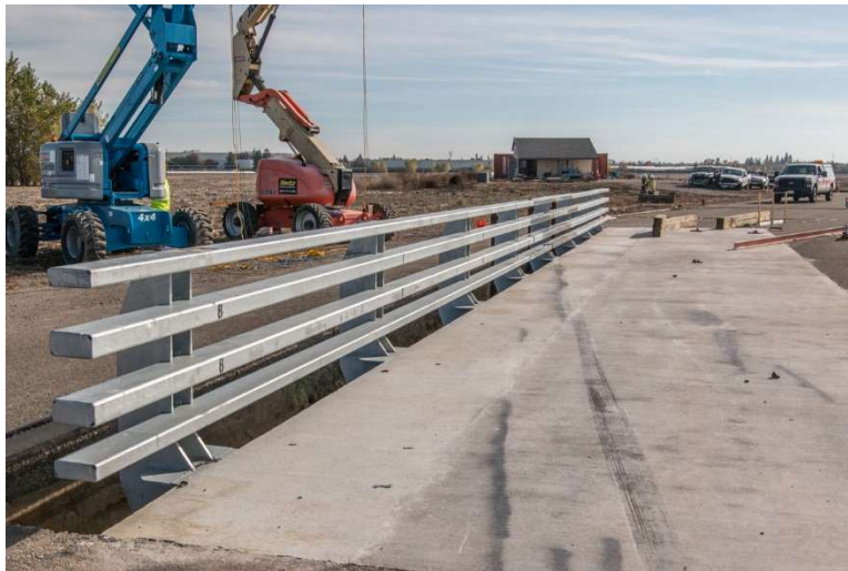
Figure 3-21. CA ST-70SM Side Mounted Bridge Rail after 1100C Vehicle
