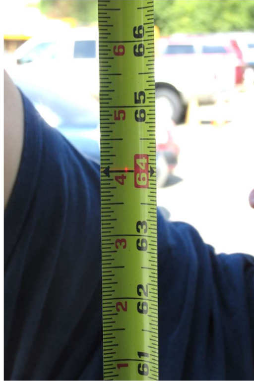
Figure 8-33. 110MASH4S16-03 Vehicle Ballast CG Height (Red Laser at 64 inches)
