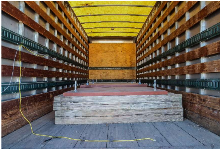
Figure 3-53. 110MASH4S16-03 Ballasts Shifted to Passenger Side
