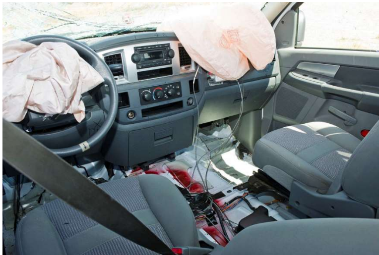
Figure 3-12. 110MASH3P15-01 Dodge Ram 1500 Airbags Deploy
