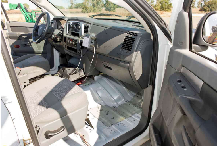
Figure 8-5. Speed Control Box Mounted to Dashboard
