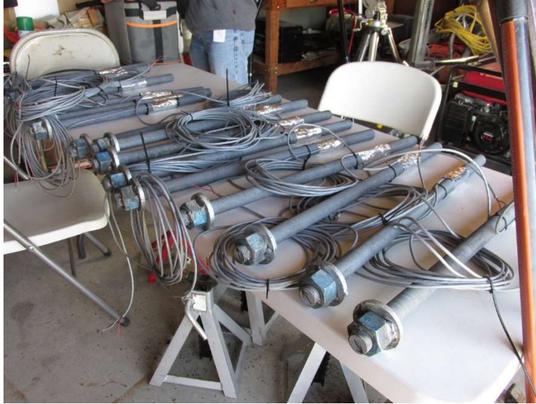
Figure 2-6. Strain Gages Installed on Anchor Rods for Posts 3, 4, and 5
