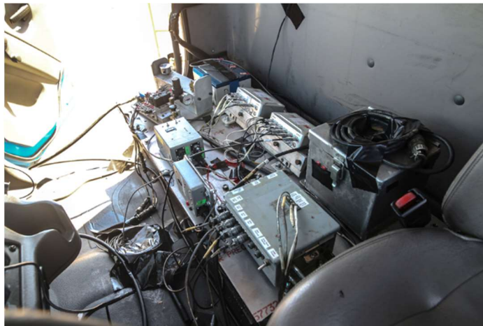
Figure 8-36. 110MASH4S16-03 Instrumentation Mounted on Passenger Seat Mount
