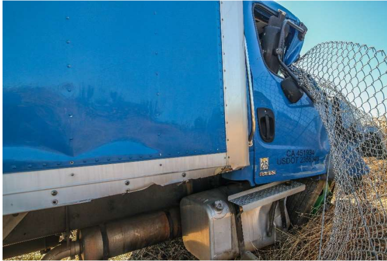
Figure 3-45. 110MASH4S16-03 Fuel Tank and Right A-Pillar Damage
