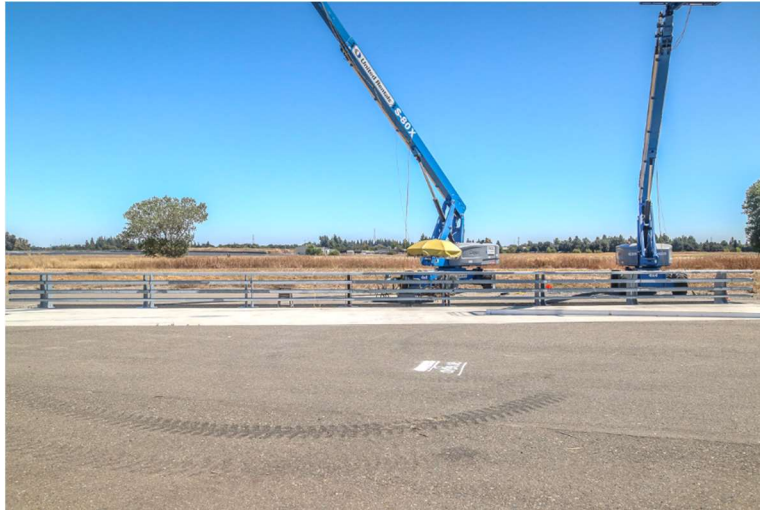
Figure 3-33. Point of Impact 60 inches (1.5 m) Upstream of Post 3
