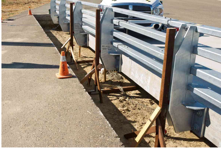
Figure 3-7. Posts 3, 4, and 5 String Pot Setup
