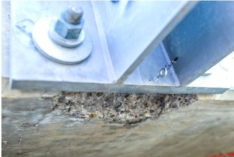
Figure 3-34. 110MASH4S16-03 Post 3 Concrete Spalling
