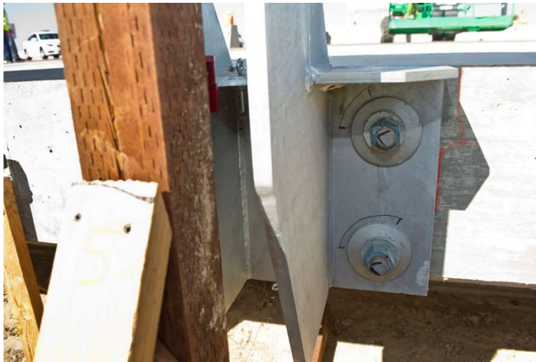
Figure 3-6. Disc Spring Installed
