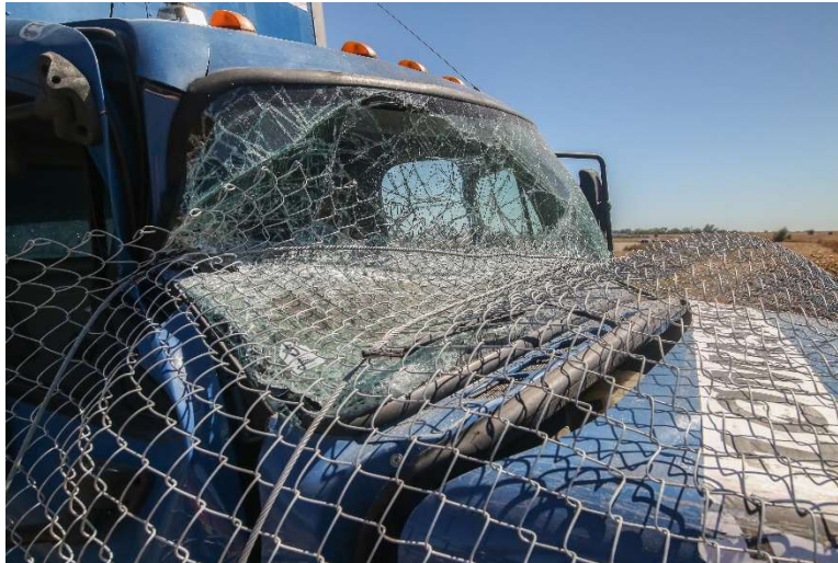
Figure 3-46. 110MASH4S16-03 Fence into Windshield
