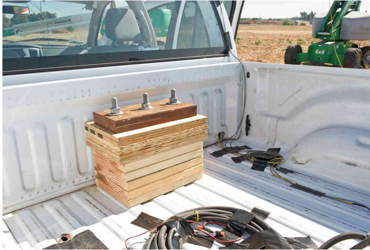
Figure 8-1. Ballast Added to Increase CG Height
