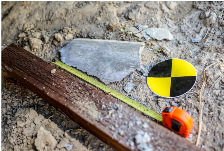
Figure 3-35. 110MASH4S16-03 Approximate Size of Spalled Concrete from Post 3
