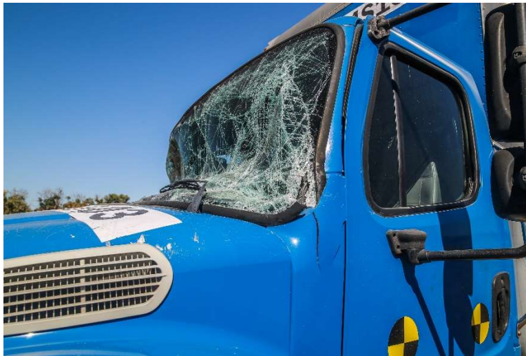
Figure 3-48. 110MASH4S16-03 Windshield Damage
