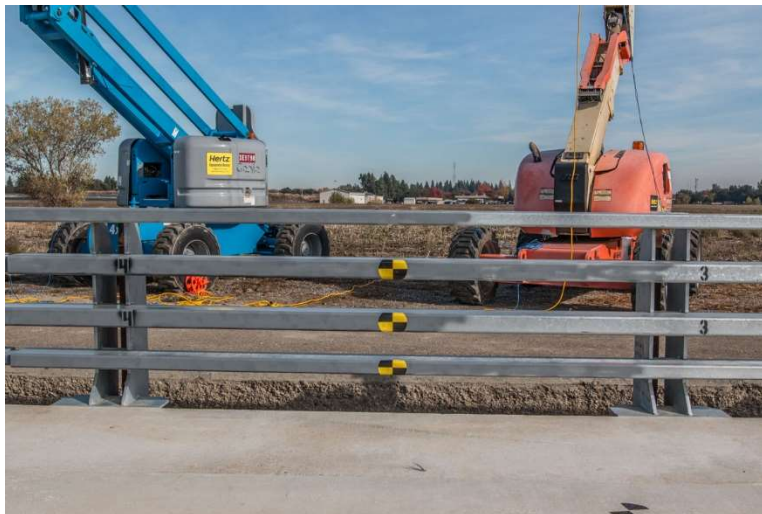
Figure 3-17. Target Point of Impact 66 inches (1.7 m) Upstream of Post 4
