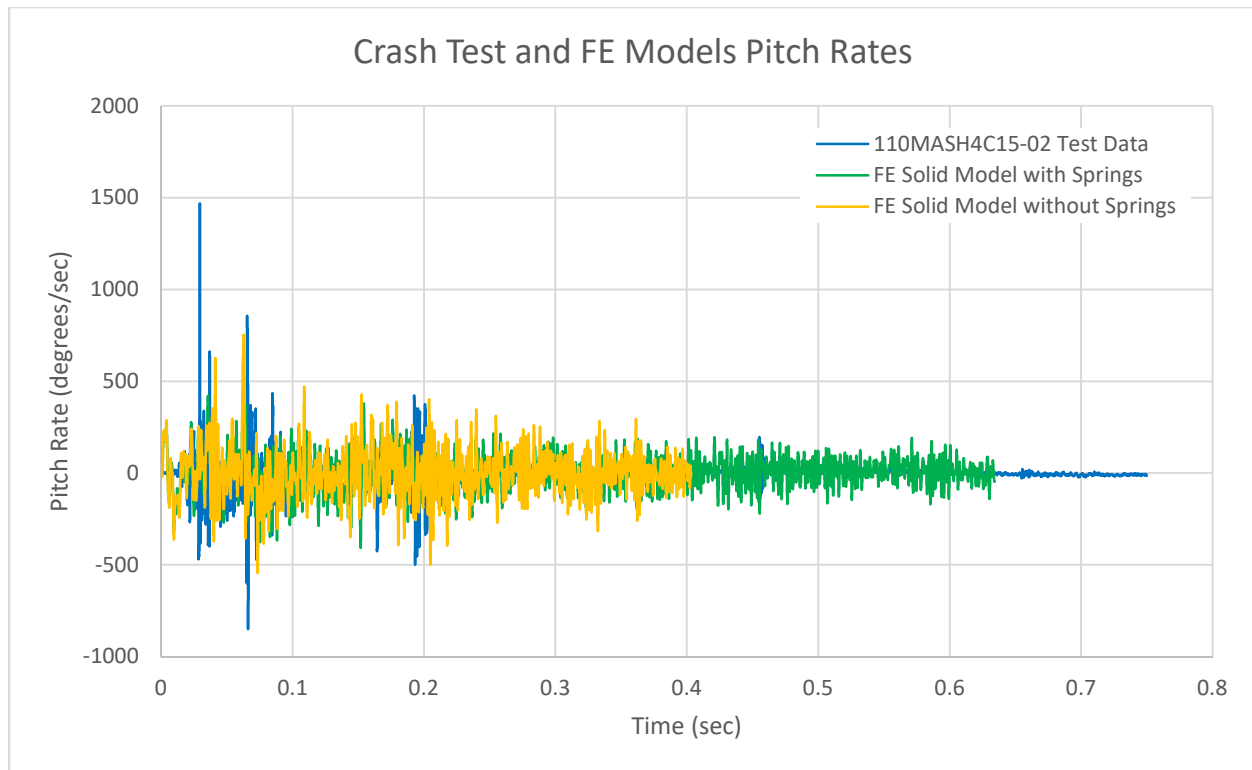
Figure 8-76. Graph of Pitch Rates for Full Scale and FE Model TRAP Results for 1100C Car
