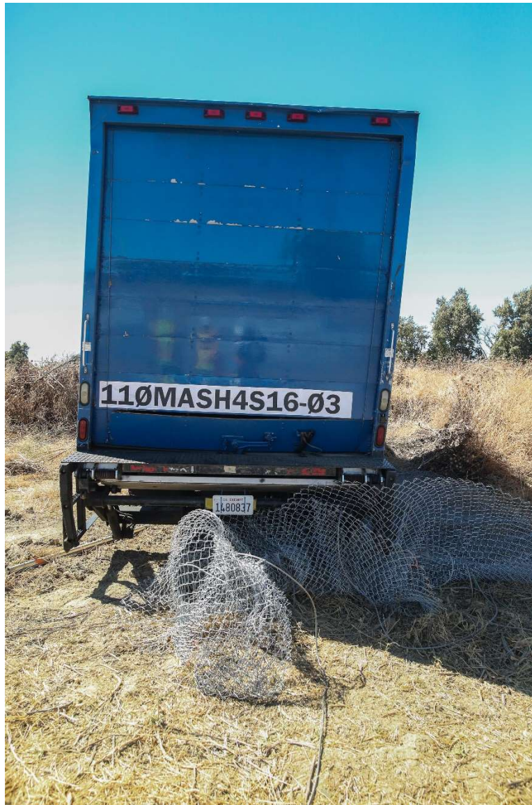
Figure 3-51. 110MASH4S16-03 Permanent Box Leaning to Impact Side
