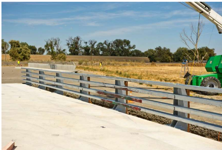
Figure 3-2. Vehicle Impact Tire Marks (Red – Front Right Tire, Green – Rear Right Tire)
