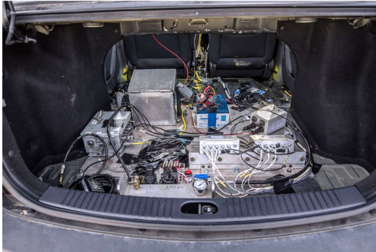
Figure 2-27. Kia Rio Vehicle Instrumentation
