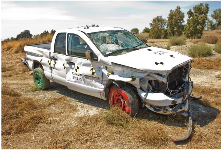
Figure 3-9. 110MASH3P15-01 Dodge Ram 1500 Damage (Side)
