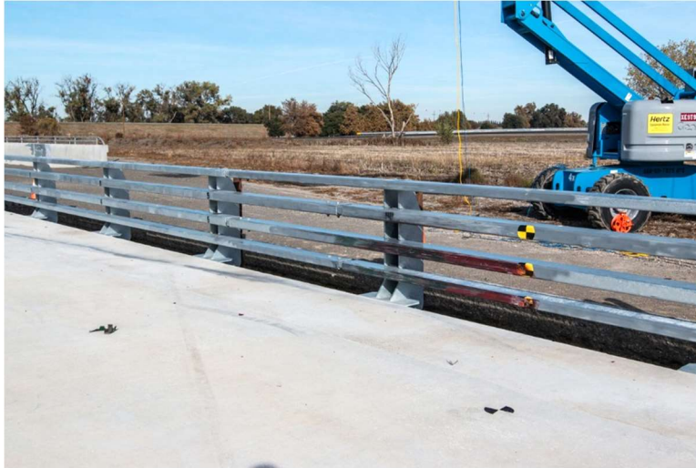
Figure 3-18. Vehicle Impact Tire Marks (Red – Front Right Tire, Green – Rear Right Tire)
