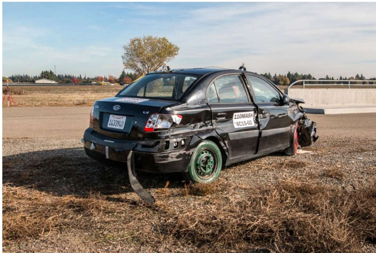
Figure 3-26. 110MASH4CP15-02 Kia Rio Damage (Rear)
