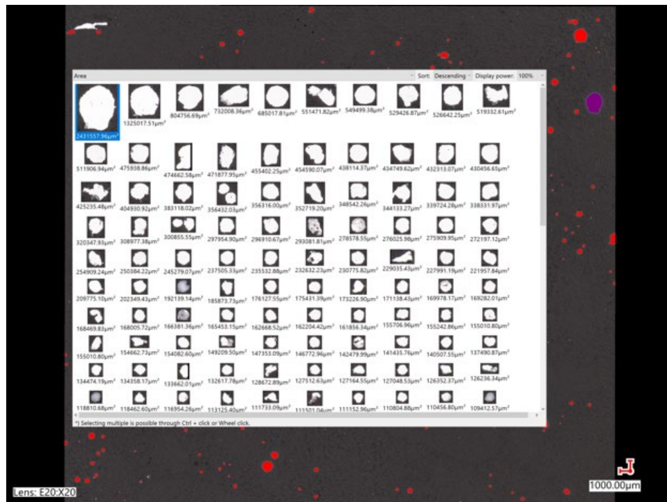
Figure 6.3 Individual Air Void Analysis Display.
