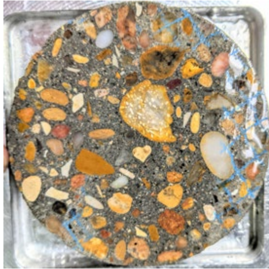
Figure A.3 Example of An Incomplete Polish.
