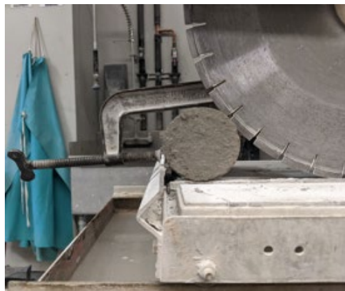
Figure 4.3 Using a c-clamp to mount the concrete sample to the saw table.
