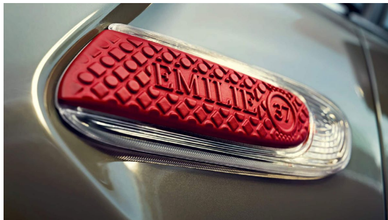
Figure 1.16: Personalized 3D printed BMW MINI scuttle collaborated with Twikit
