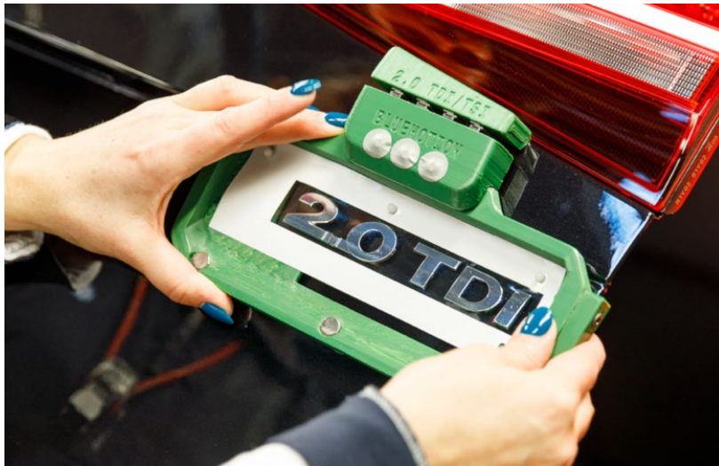
Figure 4.1: Volkswagen/Ultimaker 3D printed alignment fixture (Ultimaker)
