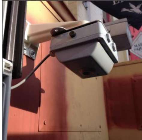
Figure 4. Eco-Counter CITIX-IR passive infrared sensor (11)
