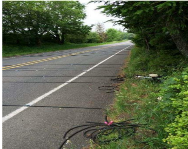
Figure 12. Pneumatic tubes stretched across road (35)
