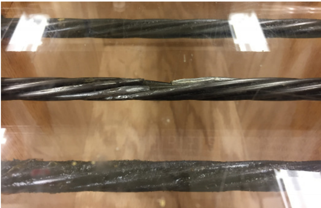
Figure 11. Strand With Gradual Section Loss
