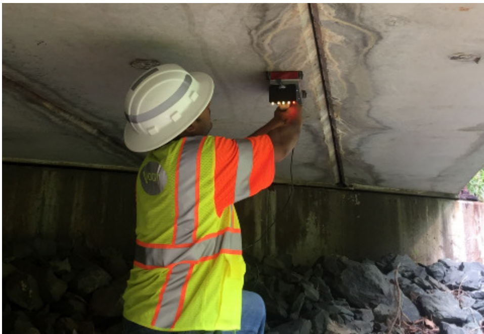
Figure 29. MFLIS Device Showing Change in Flux. MFLIS = magnetic flux leakage inspection system.
