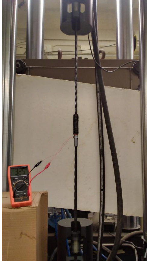
Figure 22. Tensile Loading and Magnetic Permeability Measurement
