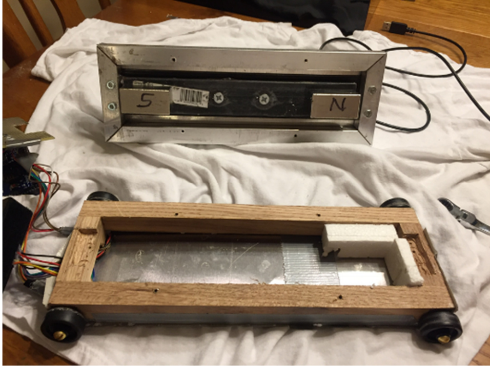
Figure 12. Disassembled MFLIS Prototype Device. MFLIS = magnetic flux leakage inspection system.
