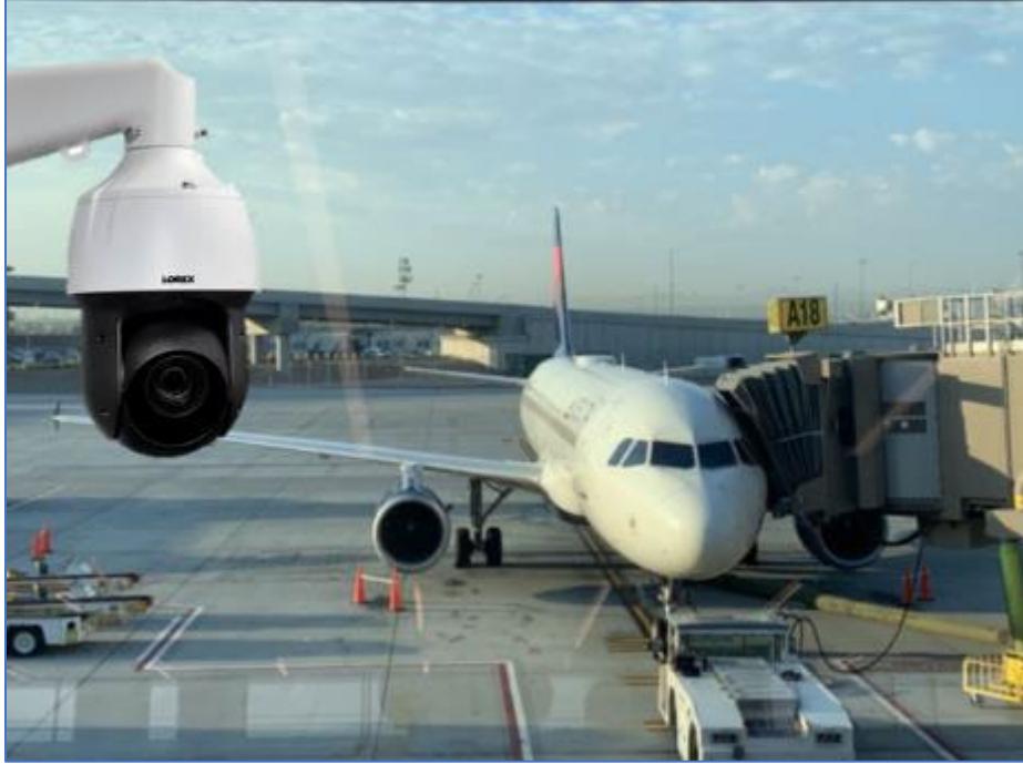
Figure 2.3 Pan-tilt-zoom camera for aircraft operation monitoring in apron area
