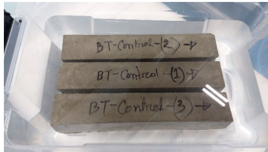
a) specimens in soak solution b) specimens stored inside an oven
