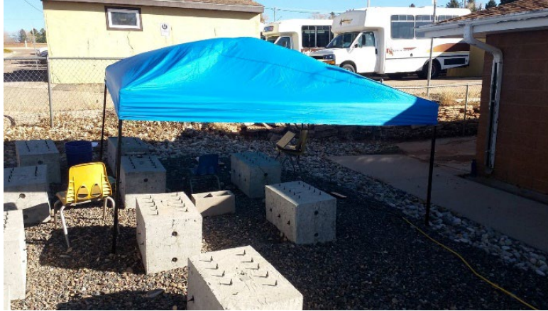
Figure 22. Photo. Exposure blocks shading prior to measurement. Source: UW Tanner Research Group.
