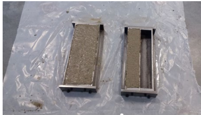
Figure 17. Photo. Min-CPT prisms inside molds. Source: UW Tanner Research Group.
