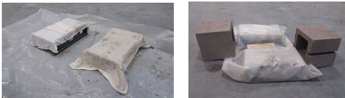
a) Prisms covered with wet towels b) Wrapped the molds with plastic sheet
