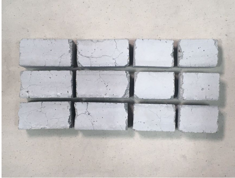
Figure 24. Mortar bars cut into sections. Source: UW Tanner Research Group.
