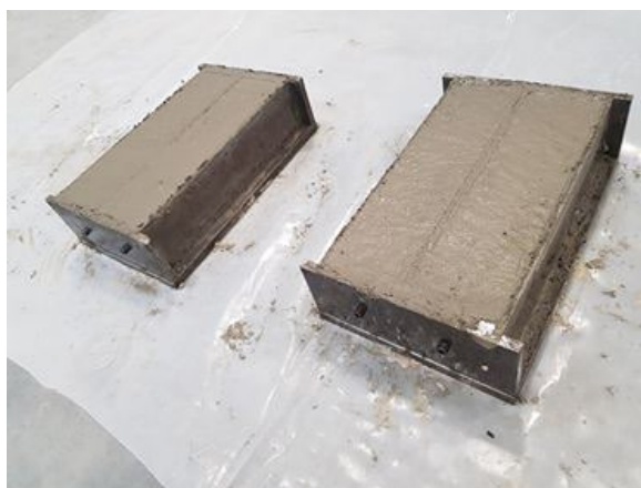
Figure 11. Photo. CPT molds with prisms. Source: UW Tanner Research Group.
