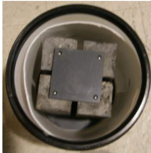
Figure 14. Photo. Storage container with supporting racks. Source: UW Tanner Research Group.
