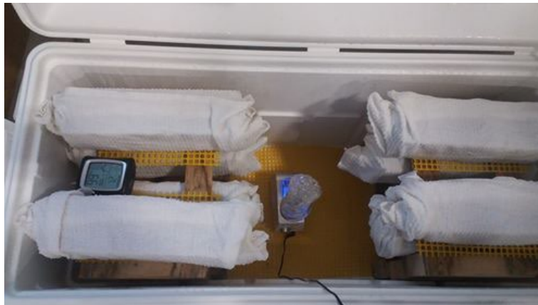
Figure 16. Photo. CPT prisms in curing chamber. Source: UW Tanner Research Group.
