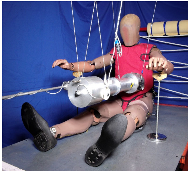
Figure 11-1. Lower thorax impact test setup
