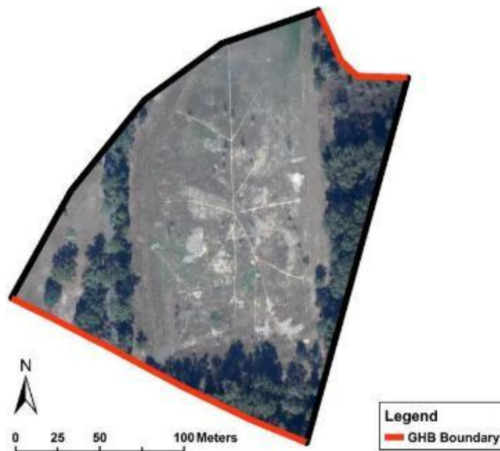
Figure 4-26. Flow boundaries applied to Layer 1
