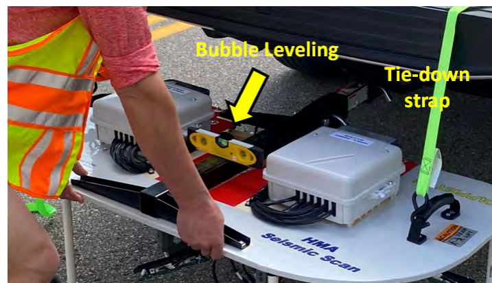
Figure 6.1.2 Procedure of leveling the receiver array frame by using a bubble-level device.
