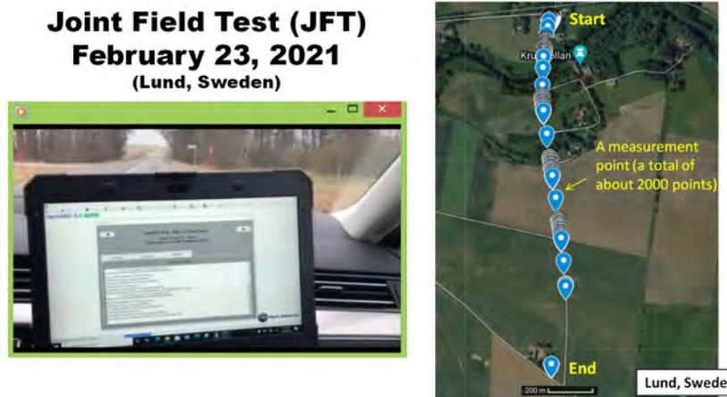
Figure 11. The on-board PS-HMA software processing data almost in real time during the joint field test (JFT) (left) and sampled data points plotted on a Google map (right).
