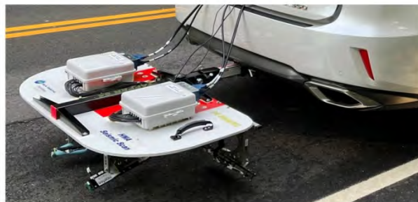
Figure 2.3 Rolling seismic pavement method that can yield multiple (1-3) data-point results per second (Ryden et al., 2019).
