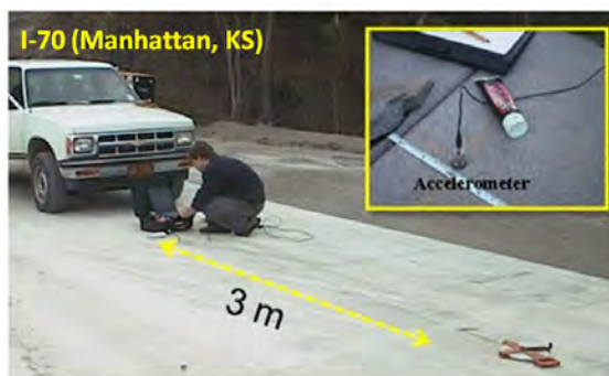
Figure 2. Seismic pavement measurement with one accelerometer (left) and analyzed Lamb dispersion image (right) (Ryden et al., 2004).
