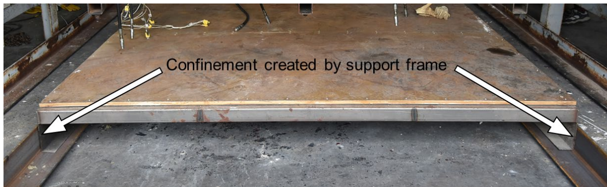
Figure 7. Test Article 2 within the built-up steel support frame
