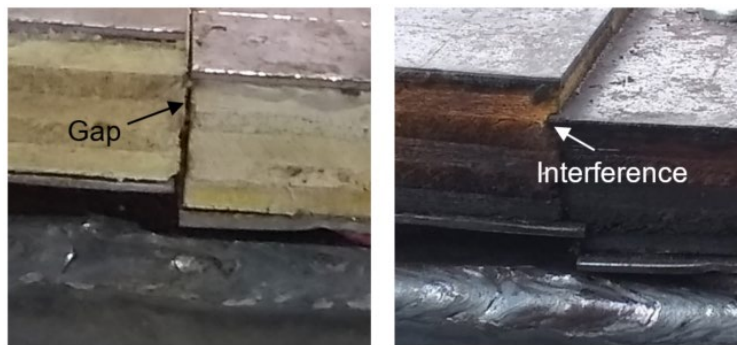
Figure 32. Observed location of ply-metal floor panel seam (left) before test with approximately 1 mm gap between panels and (right) after test with approximately 2 mm of interference between panels
