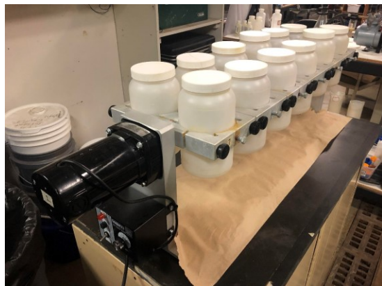
Figure 2.6. Shaker used for the preparation of soil leachate
