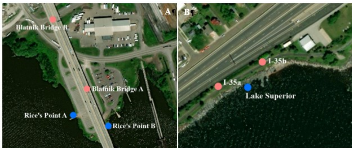
Figure 3.4. Sampling locations of Year 2 at (A) Blatnik bridge and (B) I-35. KAc runoff sites are shown in pink and receiving water body sites in blue.
