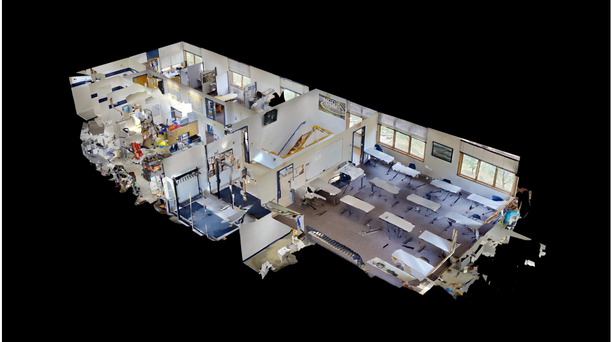
Figure 2.13 Matterport Scan from Ricoh Theta Images
