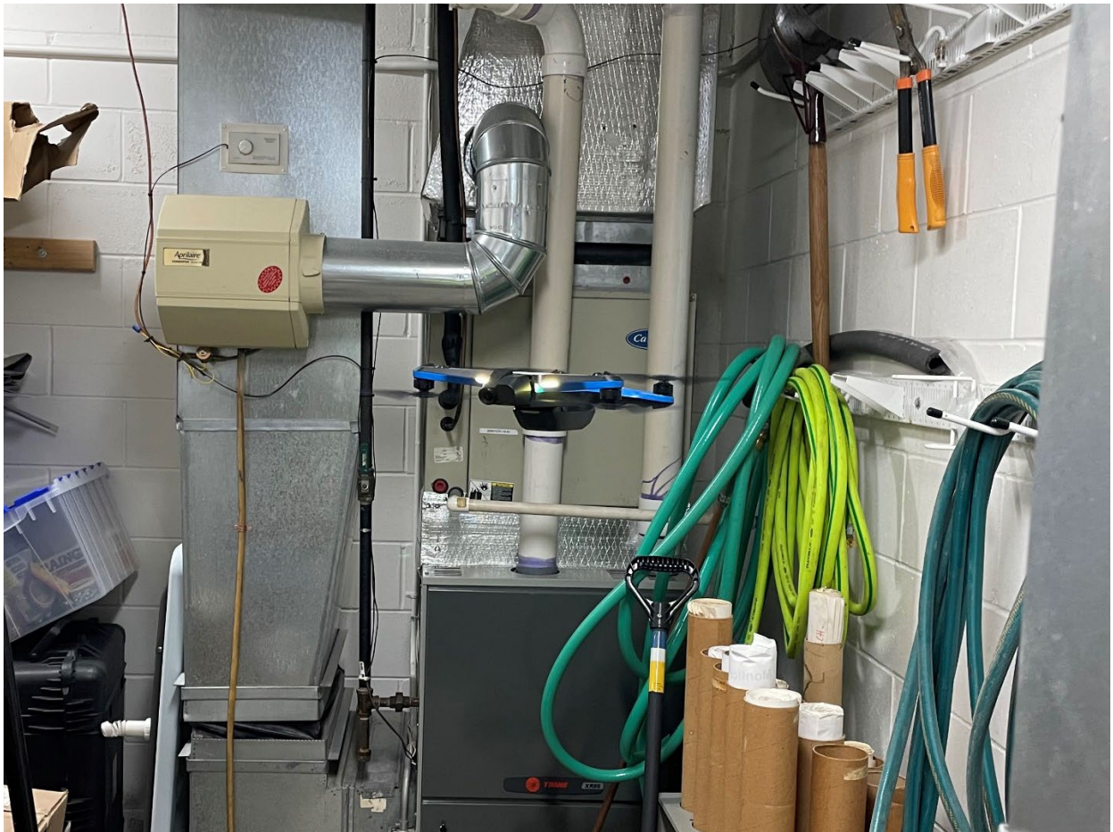
Figure 2.6 Skydio 2 Flying in Tight Area Using Obstacle Avoidance
