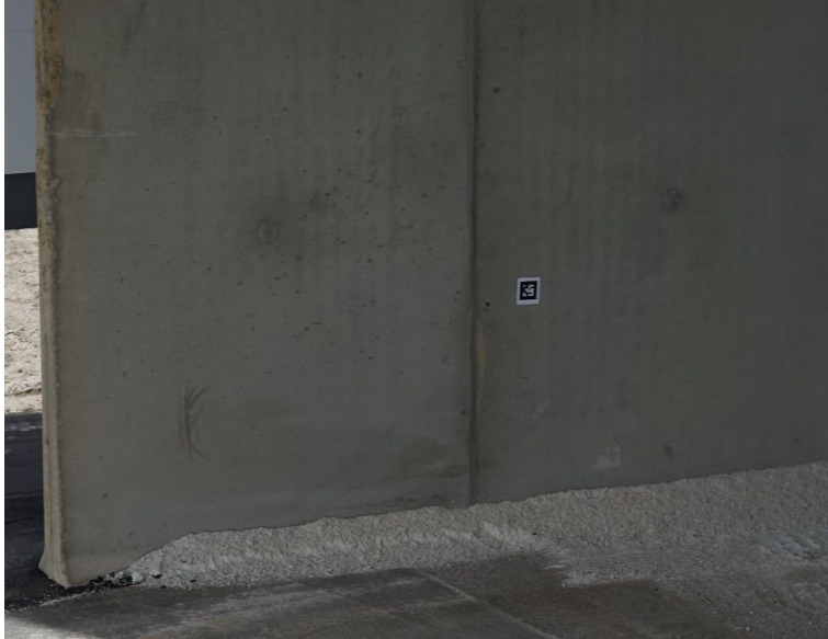
Figure 2.16 Code Target Adhered to Salt Shed Wall
