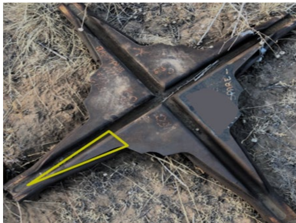
Figure 2. Crossing diamond, yellow triangular wedge shape shows the cut made
