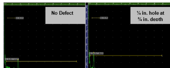
Figure 7. 2.25 MHz UT results in crossing diamond sample
