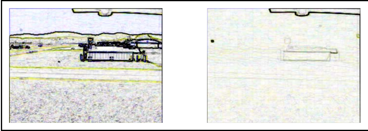
Figure 6. Edge extracted images for the Harriman airport from a clear (>20km visibility) day on the left and a low visibility (130 meter) day.
