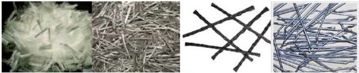
Figure 2-25 Fibers used in the (Kevern et al., 2016) study: polypropylene fibrillated fiber (left), polypropylene macro fiber (left middle), carbon fiber (right middle), and steel fiber (right).
