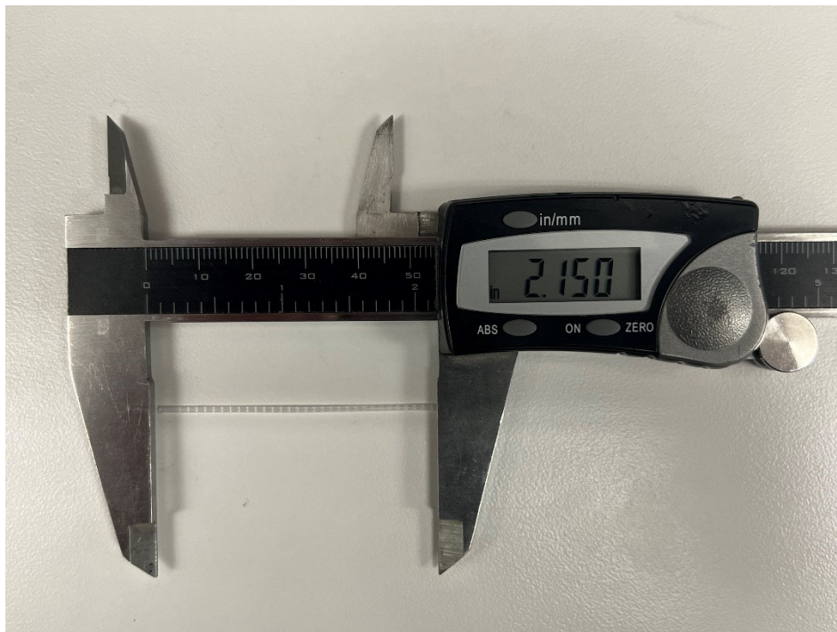
Figure 3-4. Photograph showing the length of Fiber 2 with Calipers
