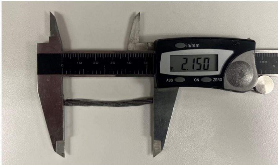
Figure 3-2. Photograph showing the length of Fiber 1 with Calipers
