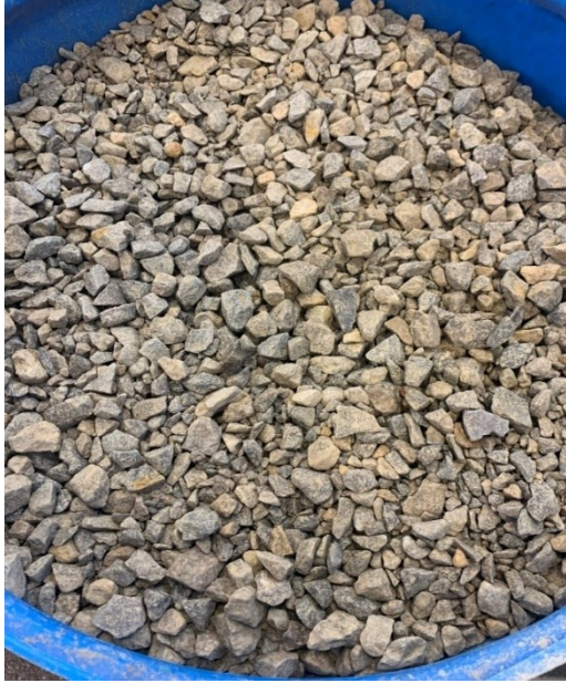
Figure 3-6. Class B Aggregates 3/4-inch and 1.5-inch (right side photograph)
