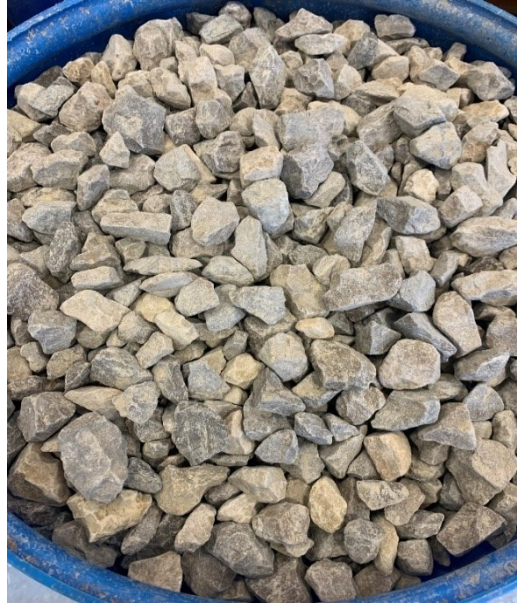
Figure 3-6. Class B Aggregates 3/4-inch and 1.5-inch (right side photograph)
