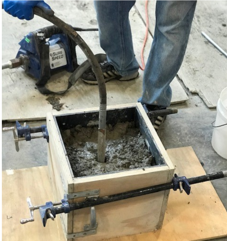
Figure 3-12. Box Test in Progress
