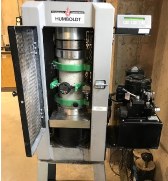
Figure 3-16. Modulus of Elasticity Test.
