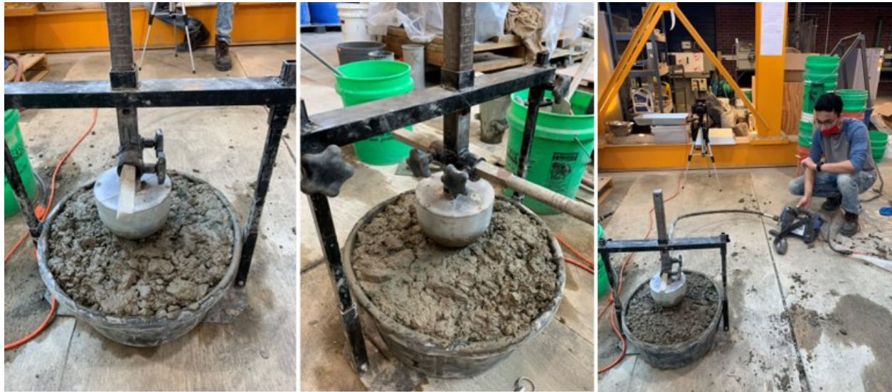
Figure 3-14. V-Kelly Test in Process
