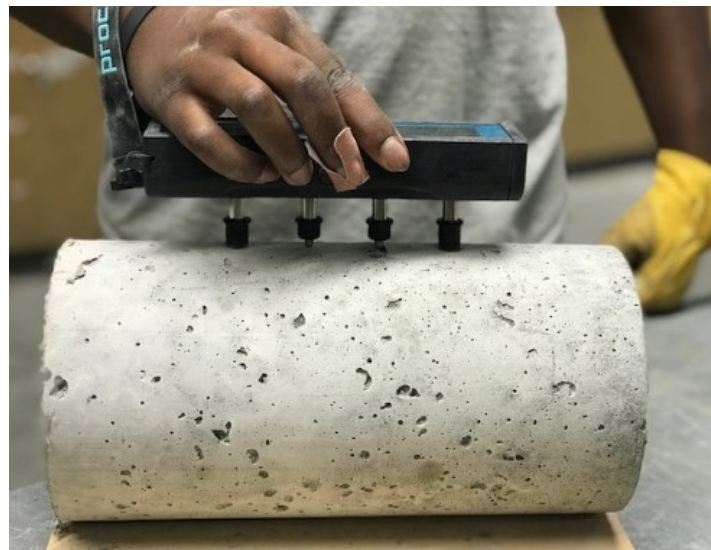
Figure 2-1 Resistivity test in progress.
