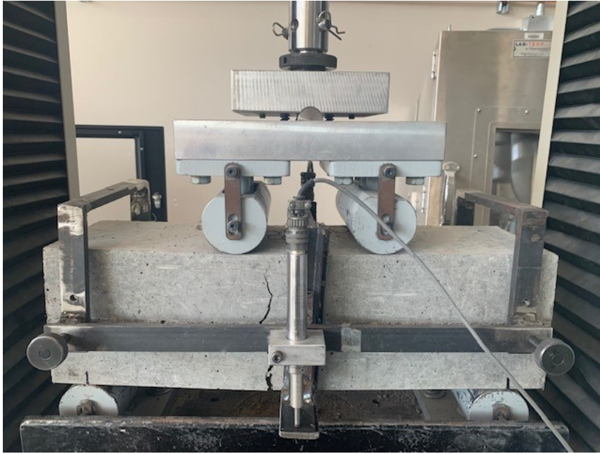
Figure 3-17. Four-Point Flexural Bend Test
