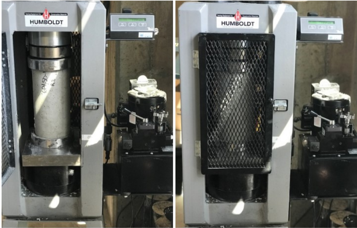
Figure 3-15. Compressive Strength Test
