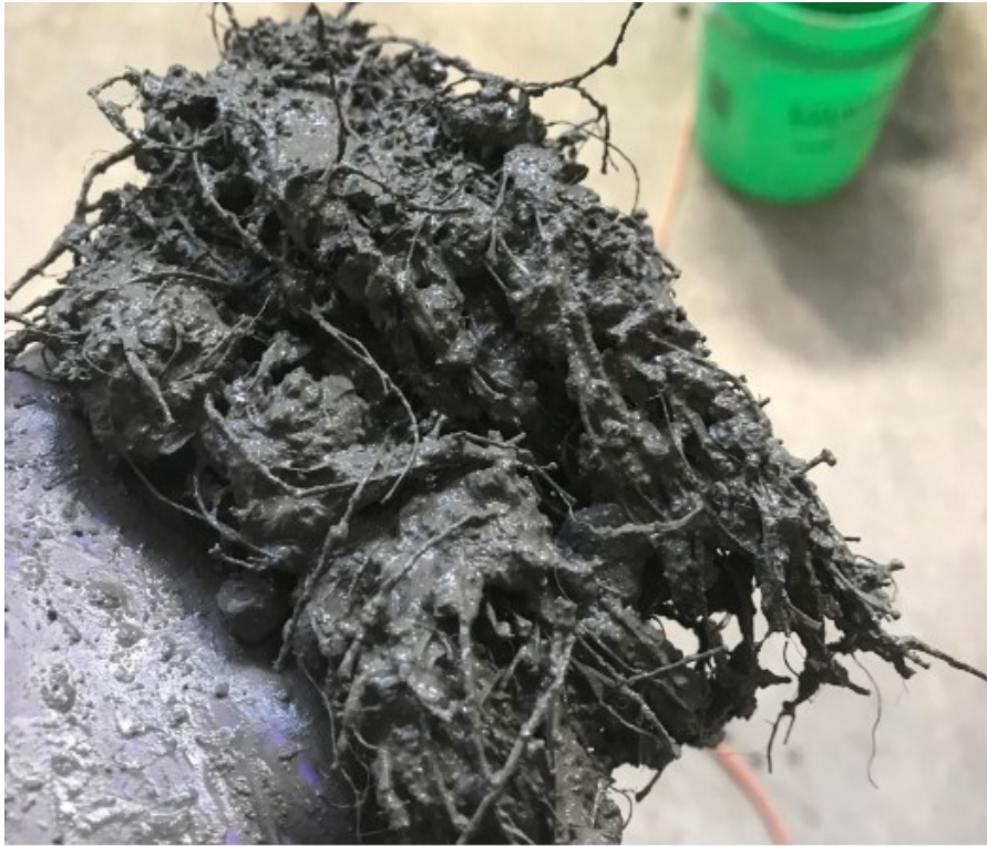
Figure 3-11. Fiber Balling of Fiber 1 (Twisted Geometry)
