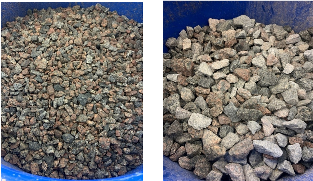
Figure 3-5. Class A Aggregates, 3/4-inch and 1.5-inch (right side photograph)
