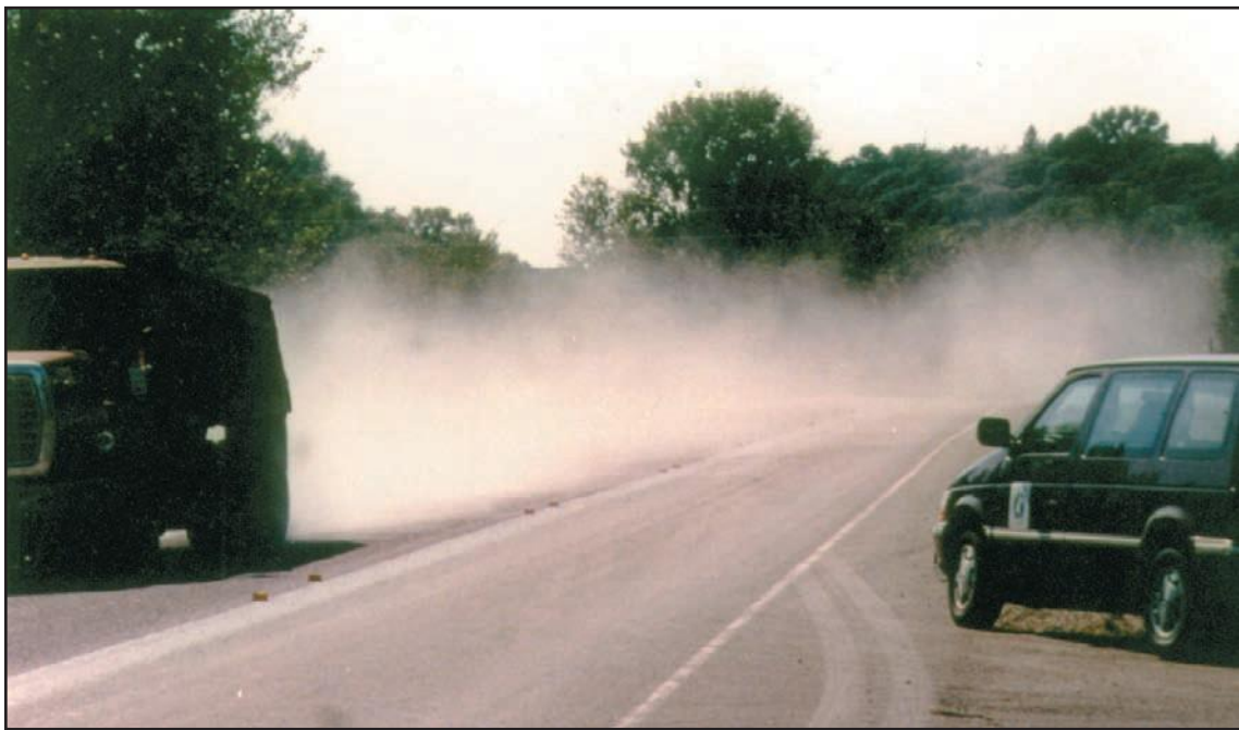
Figure 3.9.6. Evidence of a dusty aggregate
