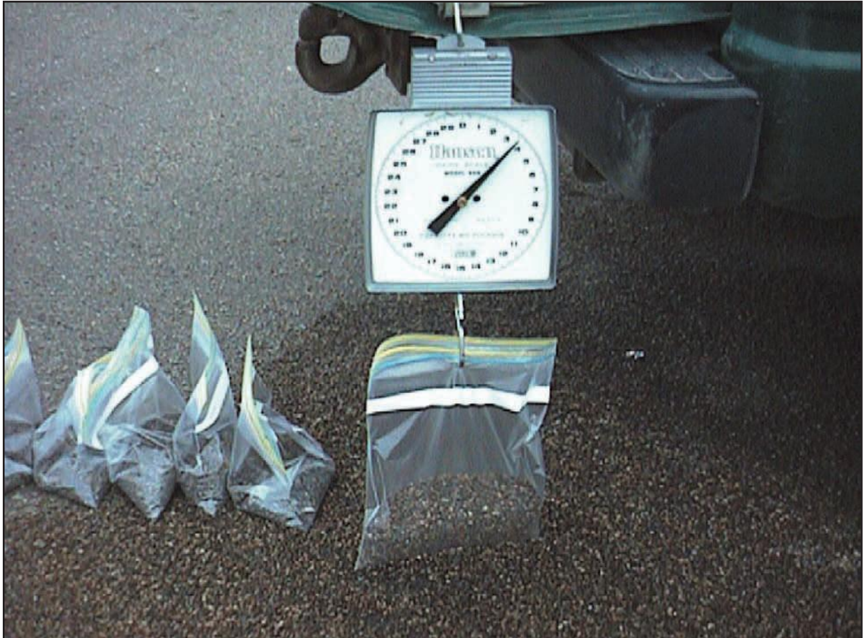
Figure 3.8.4. The contents of each bag are weighed and recorded
