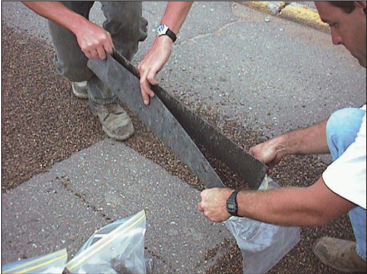
Figure 3.8.3. The aggregate on each mat emptied into plastic bags
