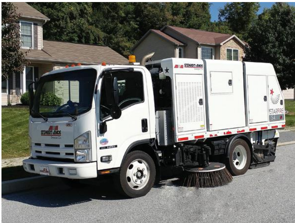
Figure 3.1.4. Pick-up sweeper typically used in urban areas
