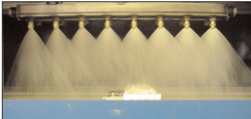
Figure 3.8.8. Spray bar nozzle showing proper alignment
