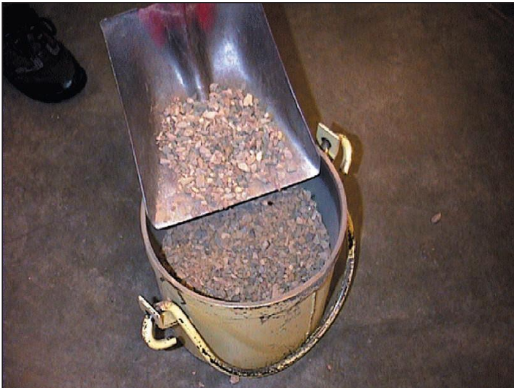
Figure 3.4.6. Loose Unit Weight Test
