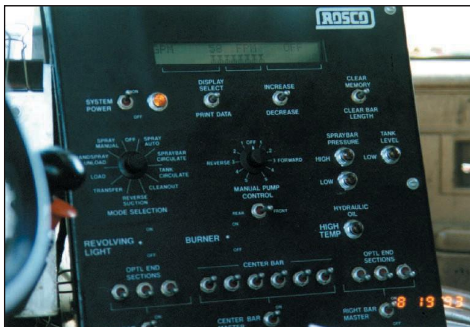
Figure 3.1.6. Computer control console of an asphalt distributor
