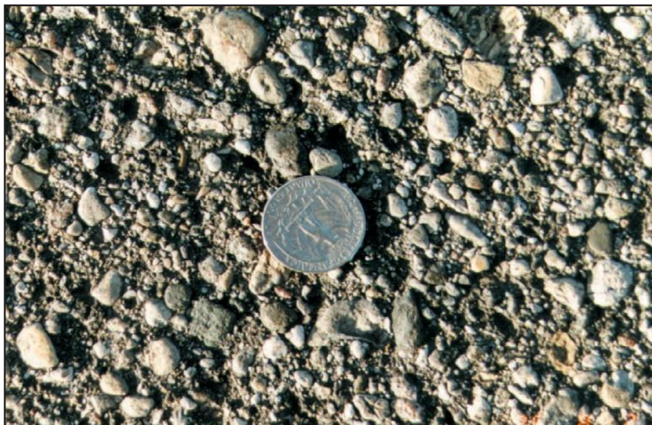
Figure 3.2.7. Example of a poorly graded round chip seal aggregate
