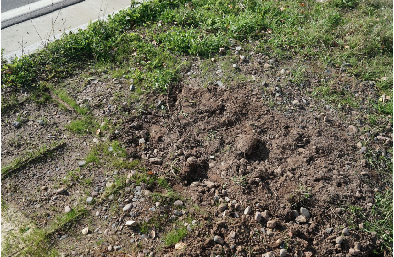
Figure 4.27 Duluth roadside research site before plot one. Numerous coarse fragments allowed the site to be highly thermally conductive containing very high daily and yearly fluctuations in soil temperatures. The planting environment generally reduced vegetation growth and persistence.
