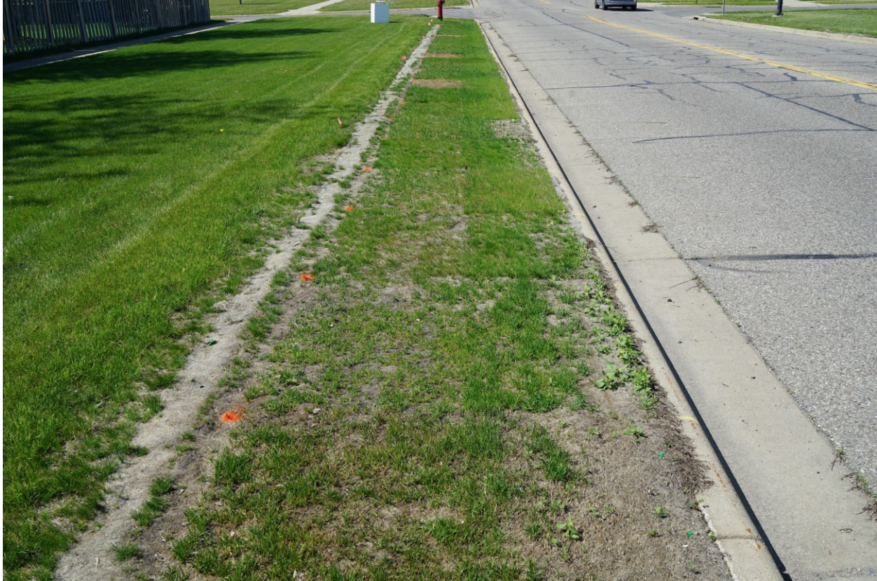
Figure 6.4 Turfgrass plots at the St. Cloud research site. This photo was taken on May 19, 2020, the first spring after seeding. Plots are showing winter damage. Differences in species abundance are shown within a plot. Plots with excessive turfgrass death near the road contained tall fescue and plots with excessive turfgrass death further from the road (see plots closer to hydrant) contained alkaligrass.
