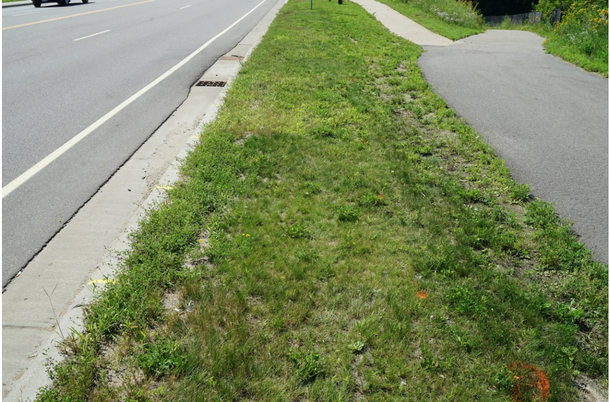
Figure 6.5 Turfgrass plots at the Grand Rapids research site classified as a poor soil quality site. This photo was taken on July 30, 2020. Plots are showing relatively sparse grass coverage with considerable volunteer legume abundance.
