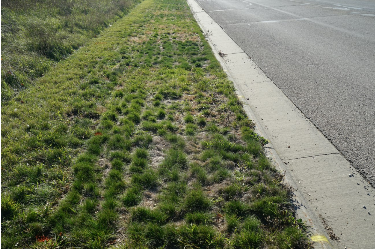
Figure 4.28 Chatfield roadside research site. Mowing during droughty conditions experienced in the summer of 2019 and 2020 resulted in some plots, especially ones dominated by fine fescues, to contain a patchwork of turfgrass vegetation.
