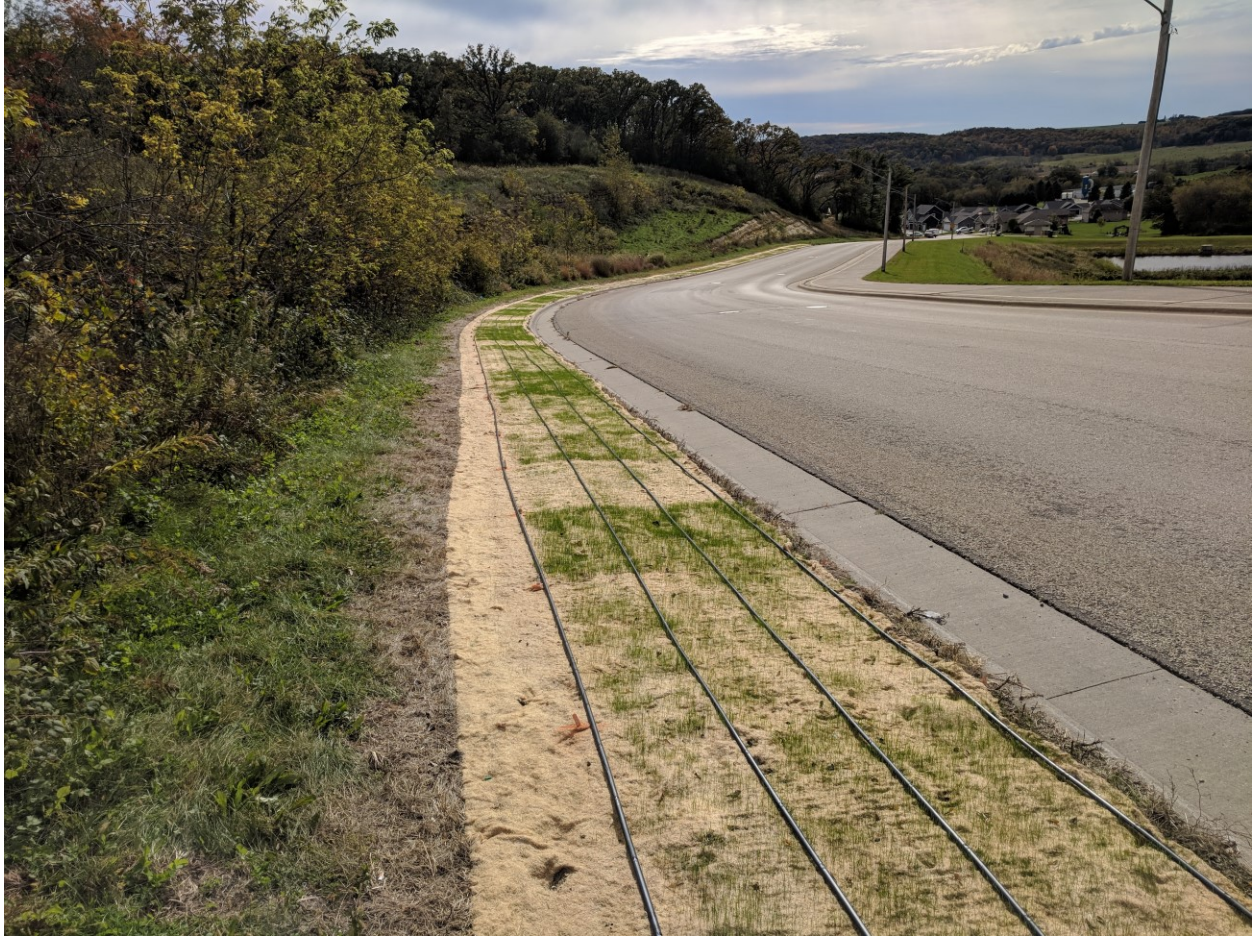
Figure 2.3 Photo showing irrigation drip lines aiding turfgrass establishment. This photo was taken at the Chatfield, MN roadside research site on Oct. 4, 2018, approximately 16 d after seeding.
