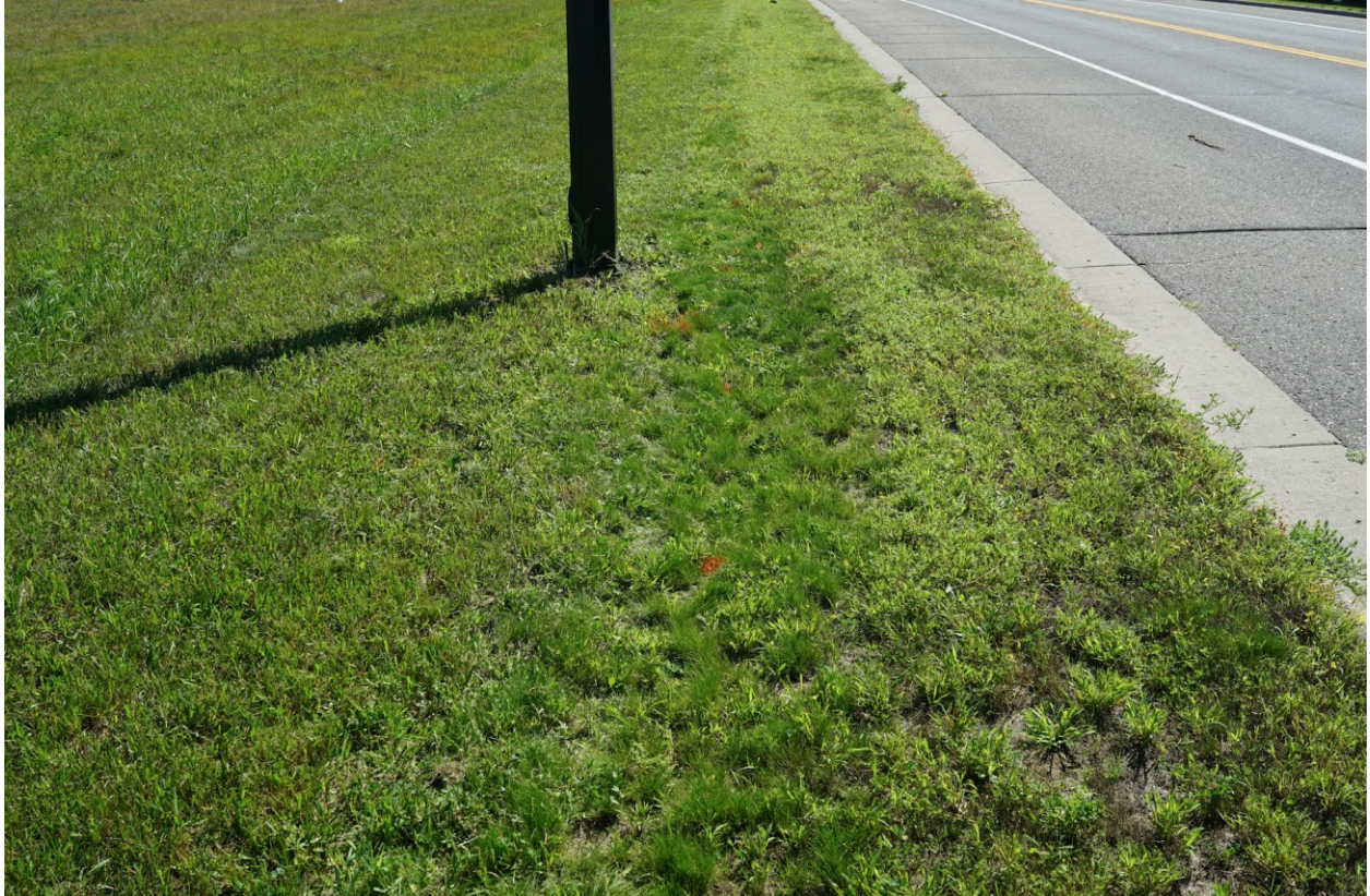
Figure 4.29 Bemidji roadside research site in the summer of 2020. Winter snowplowing showing resulted in direct damage in some plots from plow and indirect damage from grass being exposed after removal of snow. Greater turfgrass coverage near streetlight (which was not cleared) indicates that maintaining some snow cover over grass of a recent seeding can improve spring coverage.
