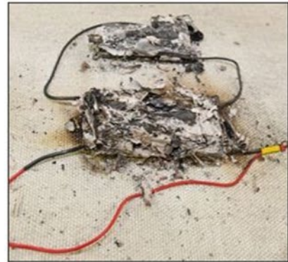
Figure 7. Peak reaction and post-test damages of each cell stack
