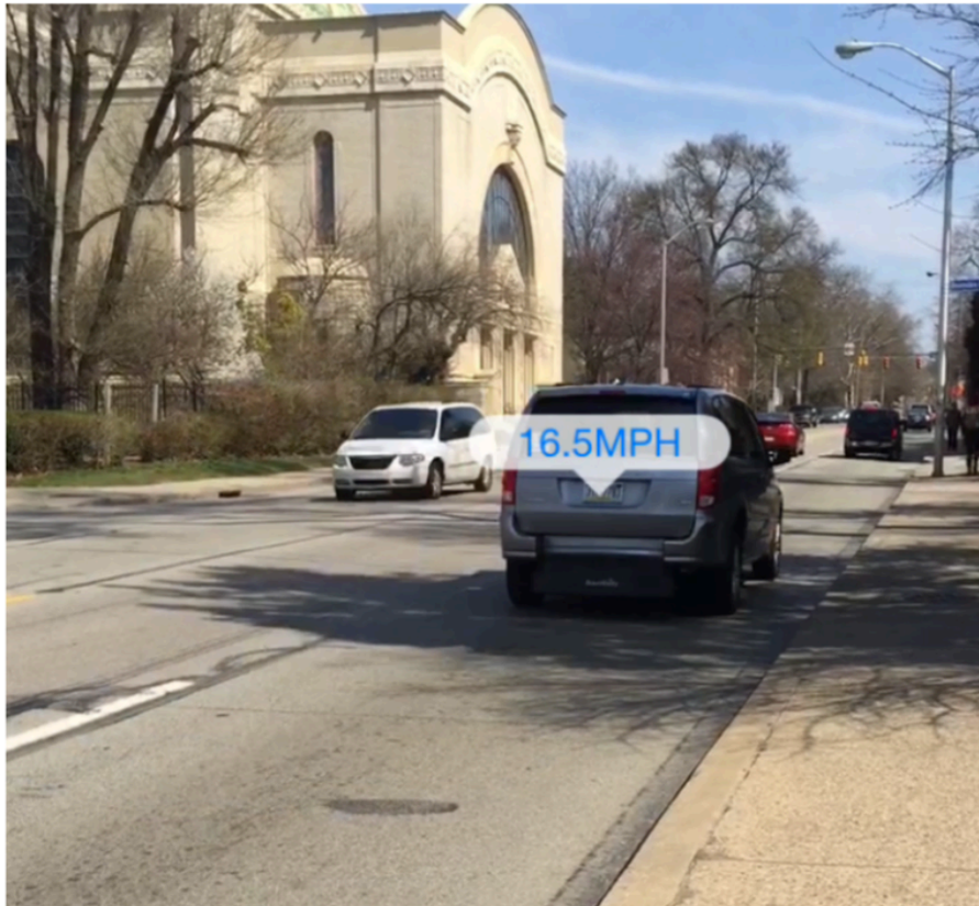
FIGURE 3. Frame of output video showing the vehicle's speed animated over its license plate.
