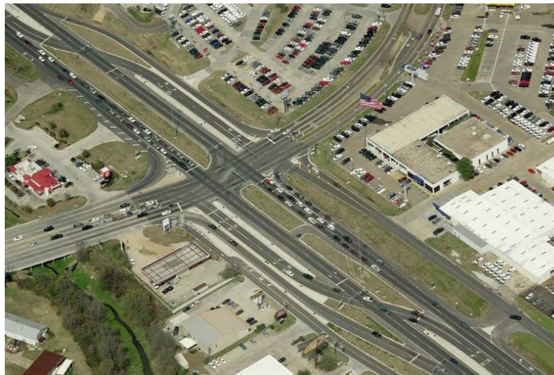
Figure 2-4: Four-legged DLT Intersection with Major Street Displaced Left Turns and Channelized Right Turns Located in Baton Rouge, LA Source: FHWA (2014)
