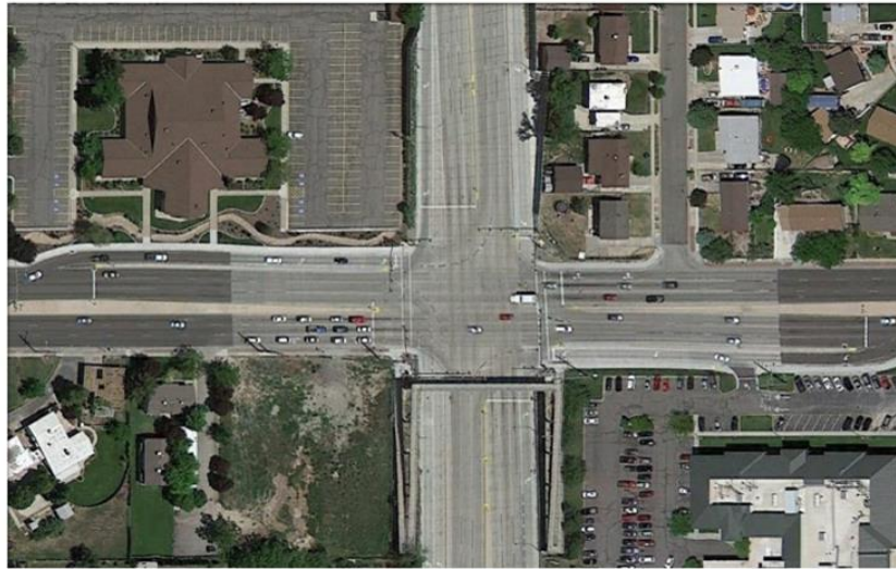
Figure 2-5: Four-legged DLT Intersection with Four Displaced Left Turns and without Channelized Right Turns Located at West Valley City, UT Source: FHWA (2014)
