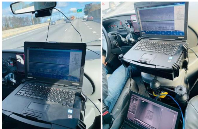
Figure 20. Photo. UGA GPR road survey control units.
