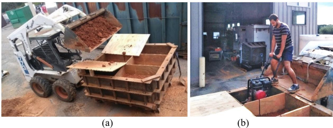
Figure 7. Photos. Sample preparation photos: (a) Soil transportation and filling testing box, (b) soil compaction
