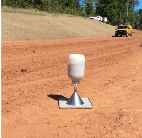
Figure 18. Photo. Sand cone test for SR 53 test section.
