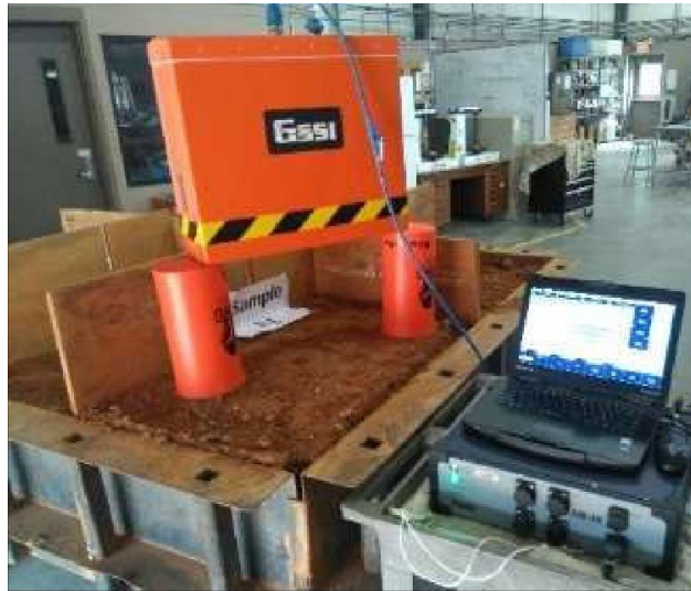
Figure 10. Photo. GPR Scanning and calibration for different samples.
