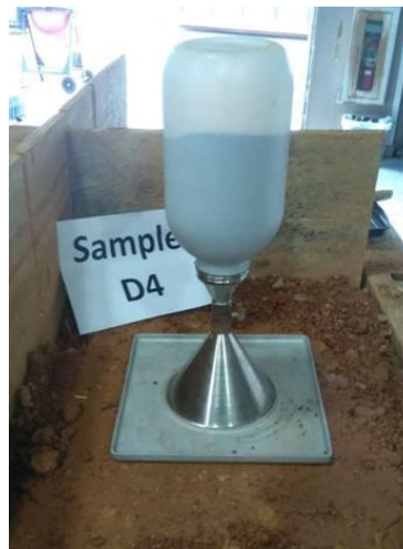
Figure 9. Photo. laboratory sand cone test.
