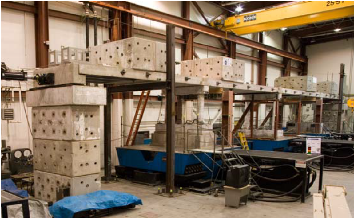
Figure 1.2. The 4-Span Prototype Reinforced Concrete Bridge
