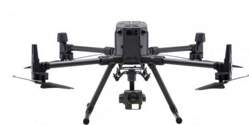
Figure 10. Photo. DJI Matrice 300 RTK
