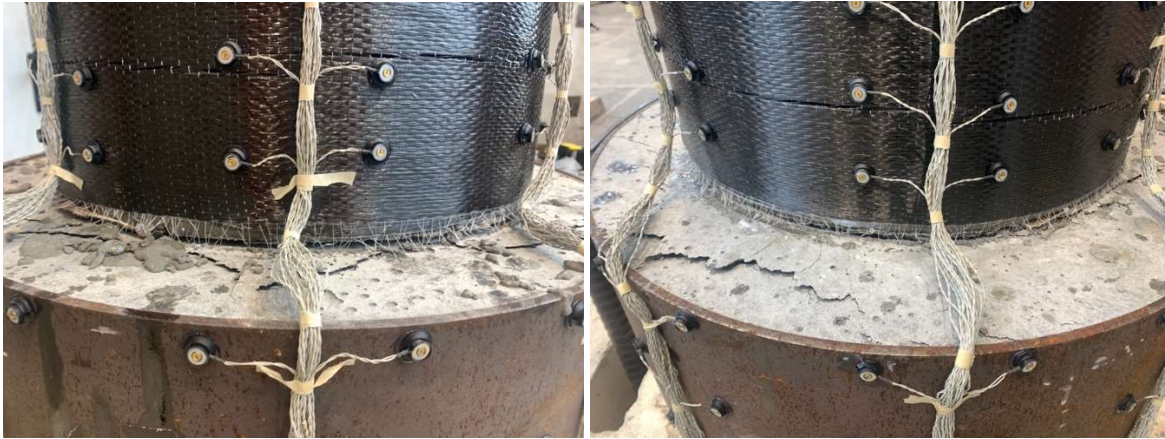
Figure 4.118: Damage Below CFRP During Ductility 3 of the North (left) and South (right) Sides.
