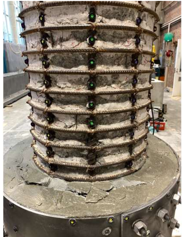
Figure 4.73: Damage after the test when all loose grout was removed of the North (left) and South (right) sides.
