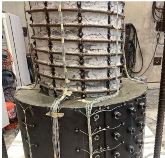
Figure 4.66 Initial damage above repair.
