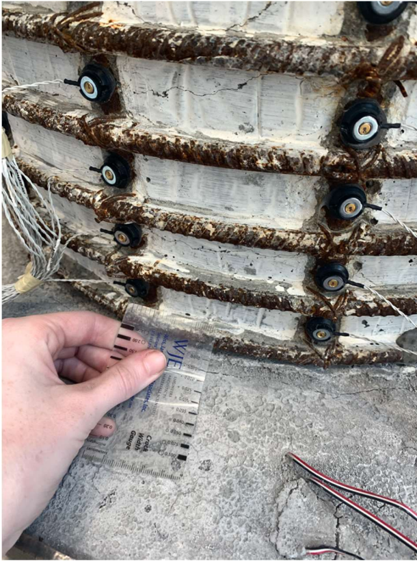
Figure 4.42: Circumferential cracks in the top of repair grout at \frac{1}{2} F_y' for the North (left) and South (right) sides.
