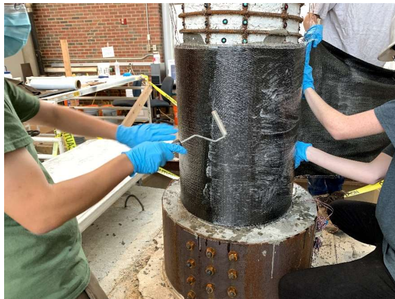
Figure 3.21: Removal of Air Voids from CFRP Wrap.
