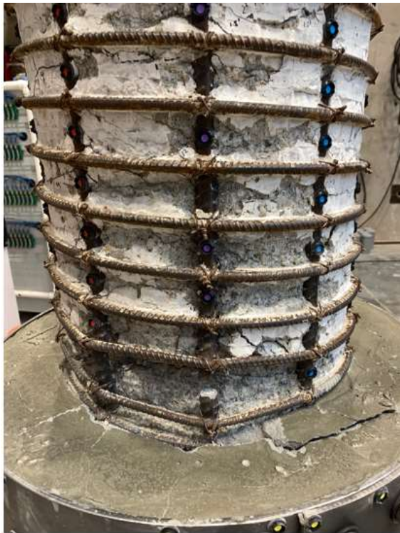
Figure 4.73: Damage after the test when all loose grout was removed of the North (left) and South (right) sides.
