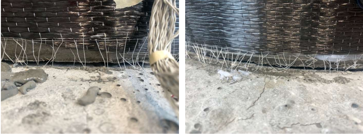
Figure 4.116: Damage Below CFRP During Ductility 2 of the North (left) and South (right) Sides.
