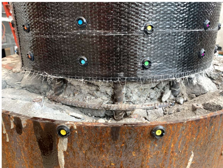
Figure 4.108: Removal of Grout to Locate Fracture Points.
