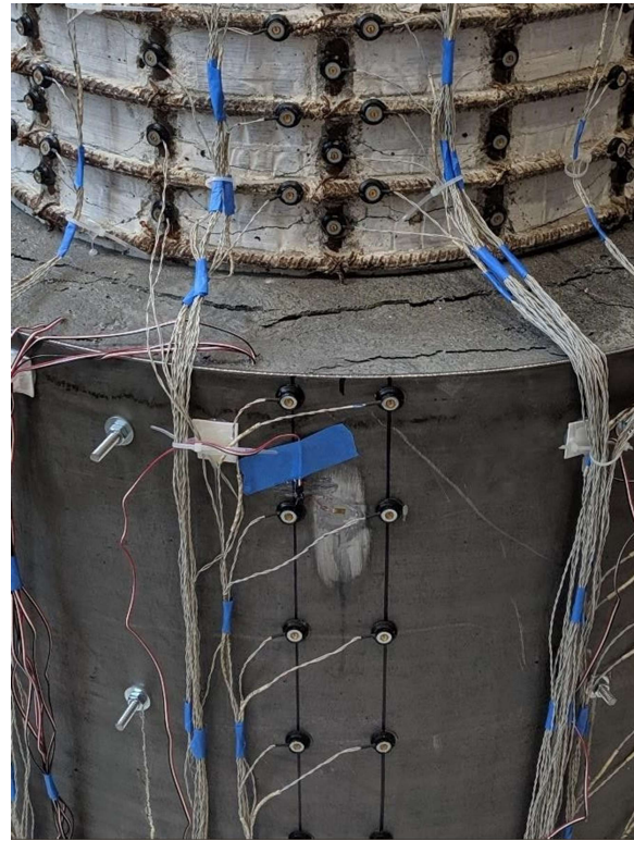
Figure 3.24: Location of Strain Gauges on Repair Bars (left) and Steel Sleeve (right).
