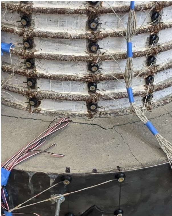
Figure 4.28: Comparison of cracking during ductility 1 for the North (left) and South (right).
