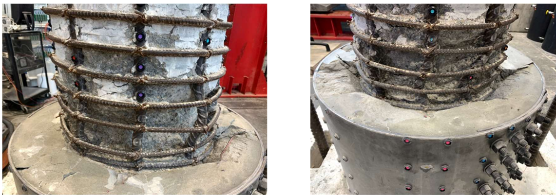
Figure 4.58: Damage Comparison after the test when all loose grout was removed of the North (left) and South (right) sides.
