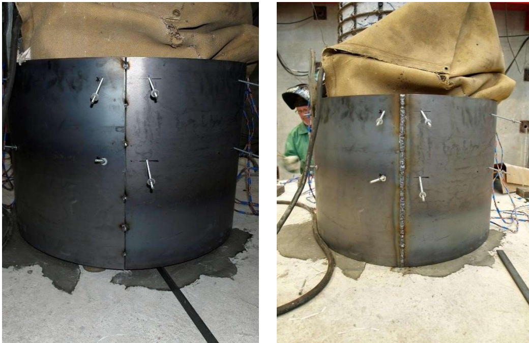
Figure 3.9: Use of Tack Welds (left) then Butt Weld (right) for Welded Connection (Krish, 2018).
