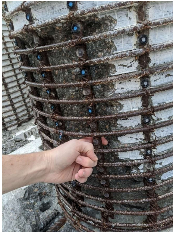
Figure 3.5: Removal of Concrete Around the Perimeter of Fractured Bars.
