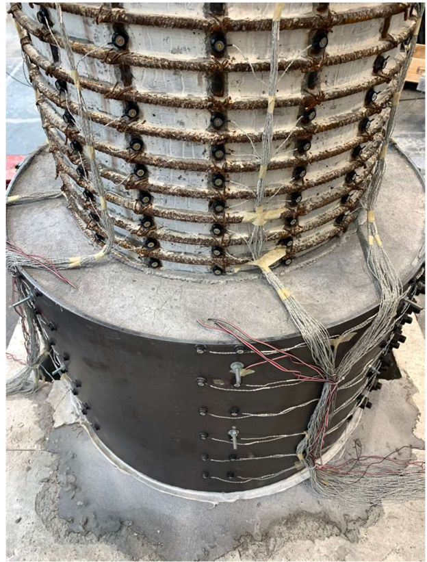
Figure 4.43: Comparison of grout cracking during ductility 1 for the North (left) and South (right) sides.
