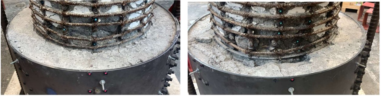
Figure 4.48: Damage Comparison after the test when all loose grout was removed of the North (left) and South (right) sides.
