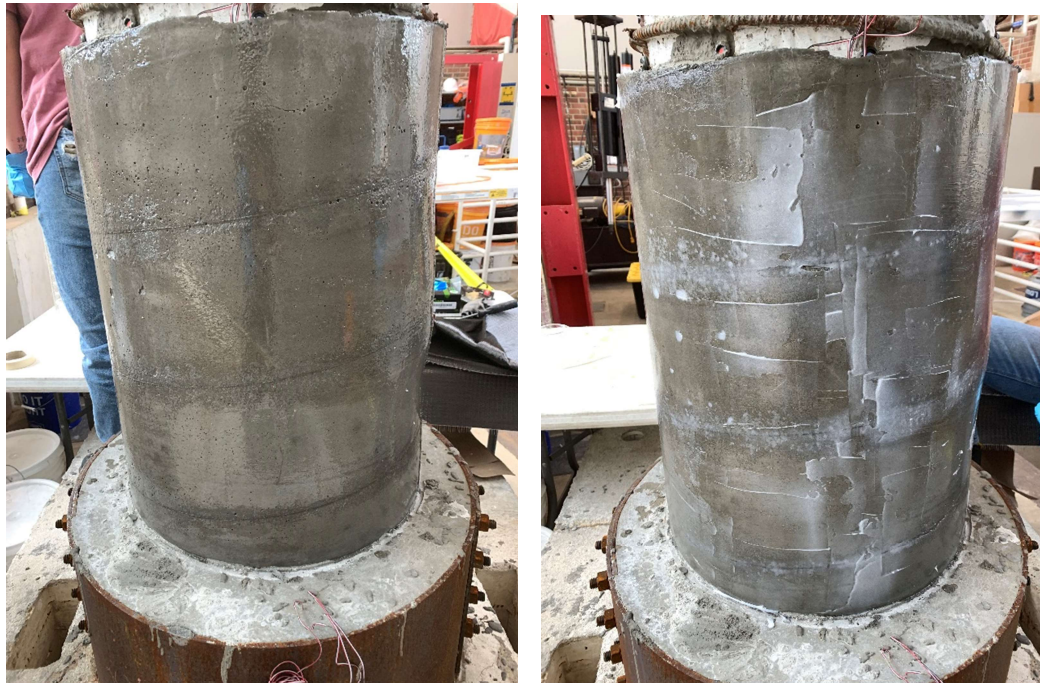
Figure 3.19: Needle-scaled Cover Concrete with Applied Primer Layer (left) and Thickened Epoxy (right).
