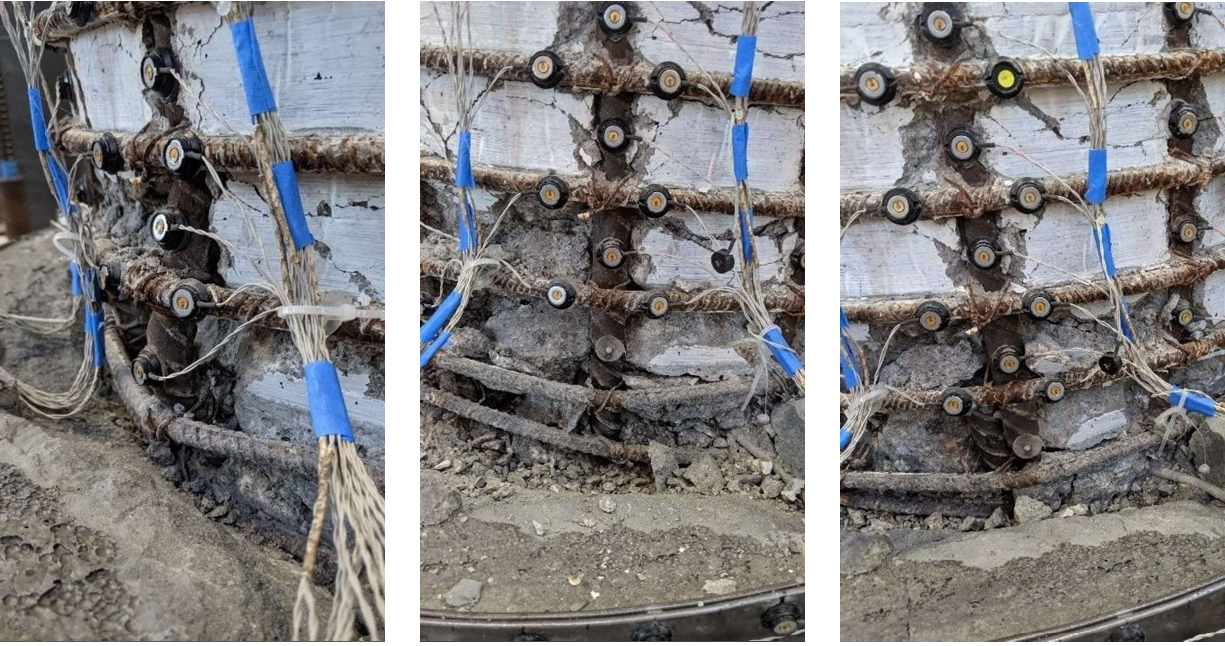
Figure 4.17: Final cycles of N6 showing (left) buckling, (middle) fracture, and (right) next compression cycle.
