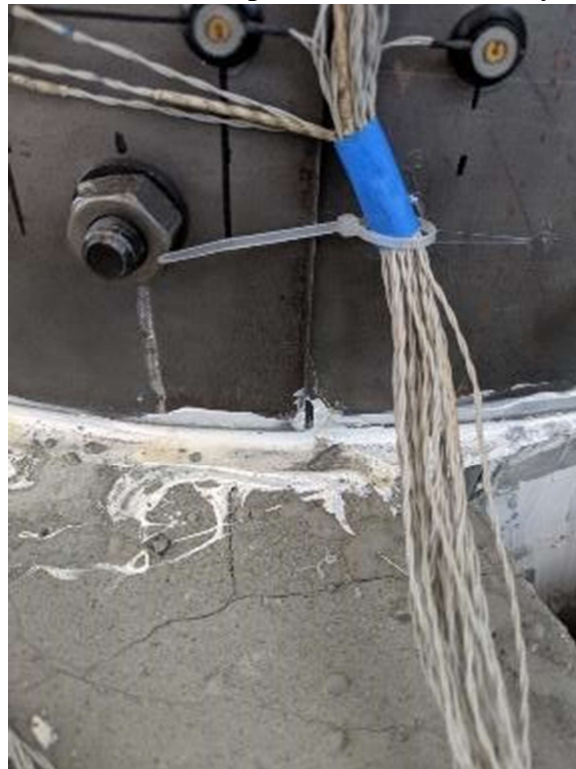
Figure 4.7: View of silicone sealant where gap formed due to plates slipping.
