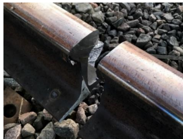
Figure 1. Rail Gap After a Rail Break Test
