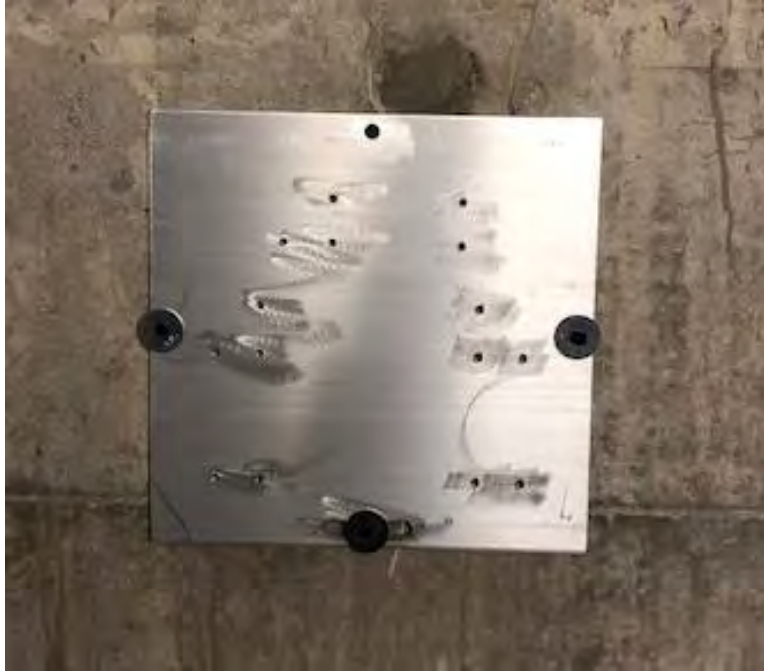
Figure 3-5: Aluminum plate for mounting accelerometers
