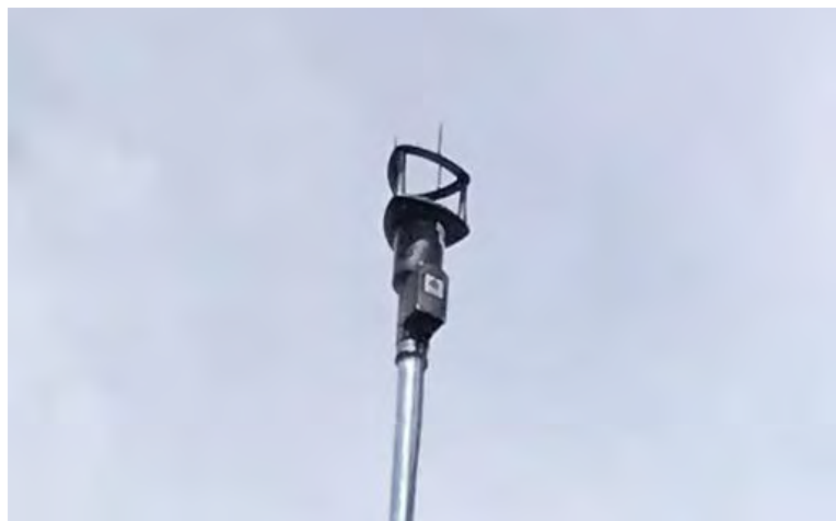
Figure 3-16: Ultrasonic anemometer installed at utility shed
