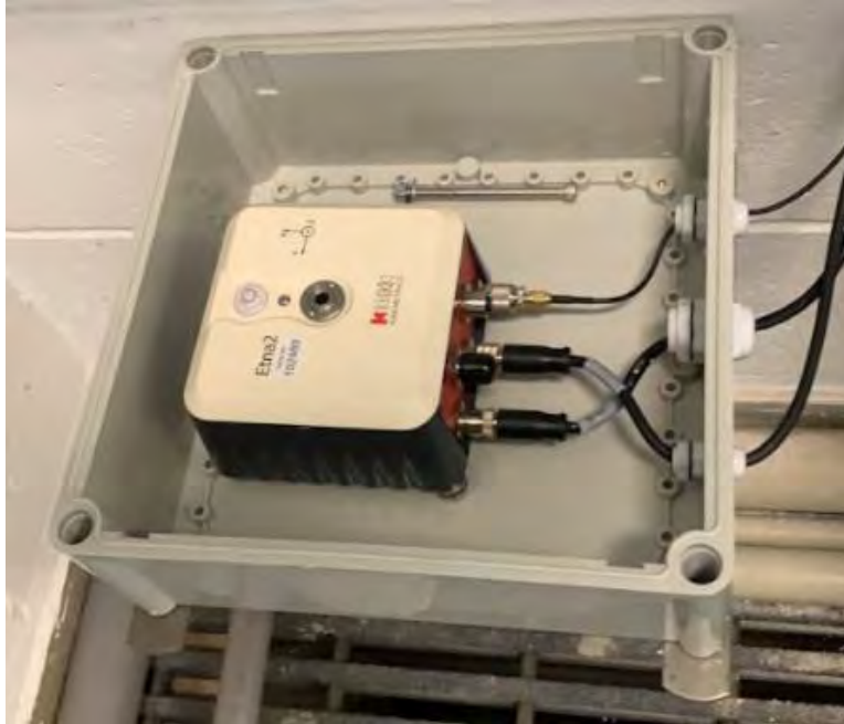
Figure 3-19: ETNA 2 accelerograph and protective case
