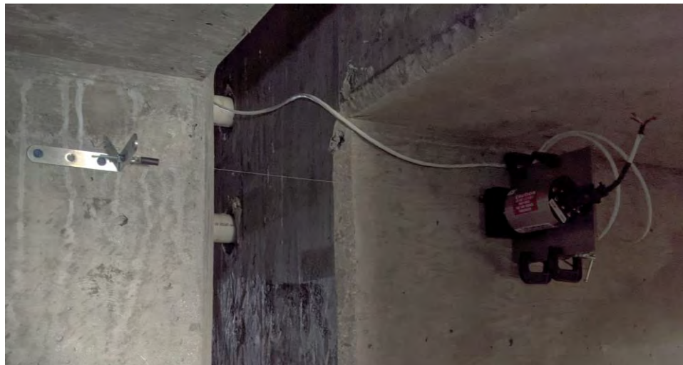
Figure 3-13: Example of potentiometer installed at Hinge 1
