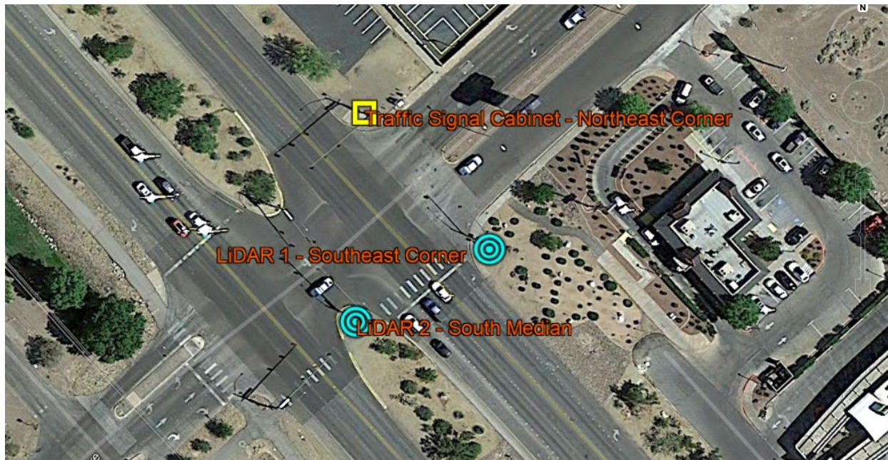
Figure 2-3 Locations of LiDAR sensors and traffic signal cabinet at S Boulder Hwy and Texas Ave
