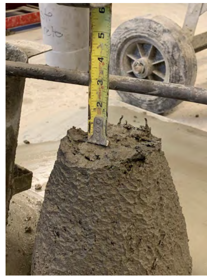
Figure 4.14 Comparison of Lincoln-Ref and FRC mix stability and appearance
