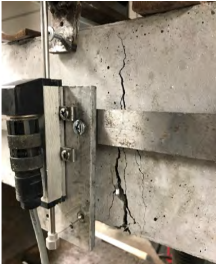
Figure 4.21 Typical FRC crack at conclusion of test
