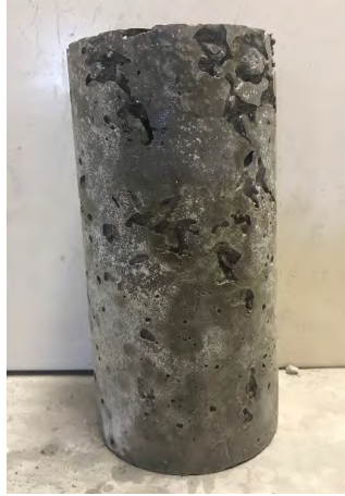
Figure 4.16 Example casted cylinder specimen with inadequate paste
