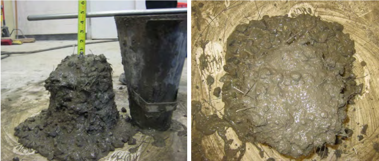
Figure 4.2 Effect of excessive water reducer on stability
