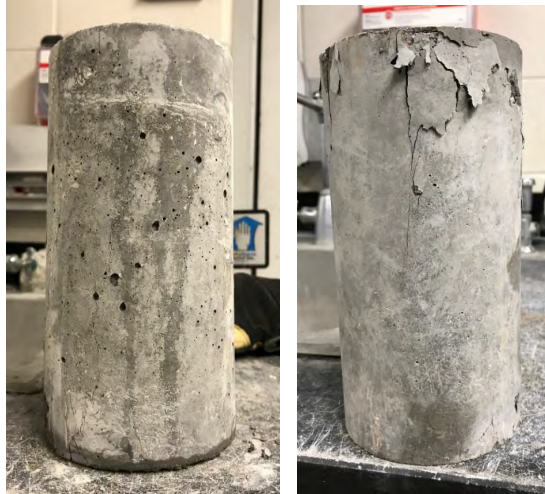
Figure 4.18 Typical compression cracks of FRC cylinders after failure
