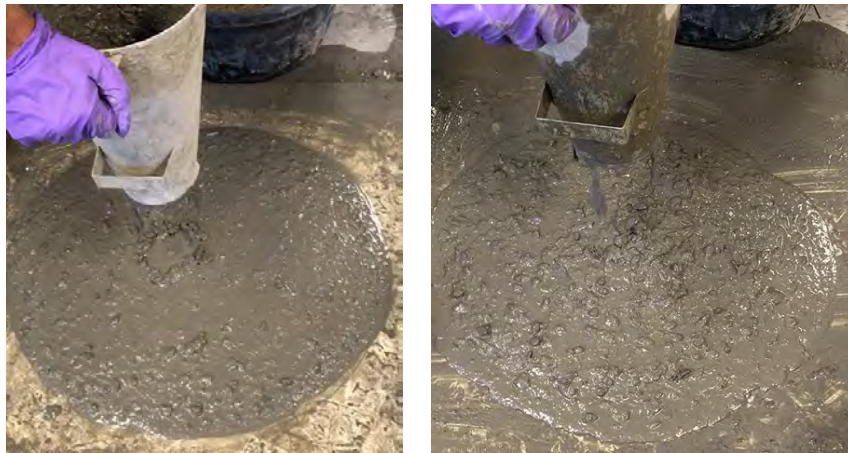
Figure 5.4 SHPC4 consistency before and after adding fibers
