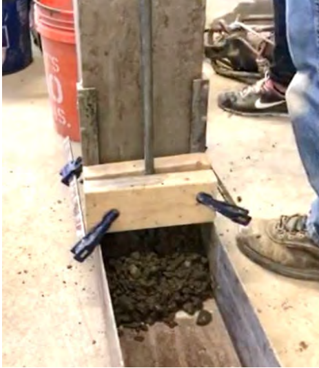
Figure 4.13 Comparison of LV-Ref and LV-FRC stability during vibrated L-Box test
