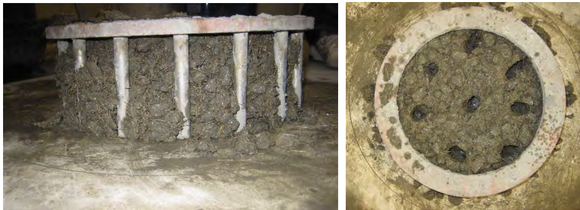
Figure 4.1 Example of FRC made with an insufficient paste
