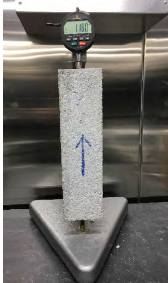
Figure 3.19 Free shrinkage specimen length measured by length comparator
