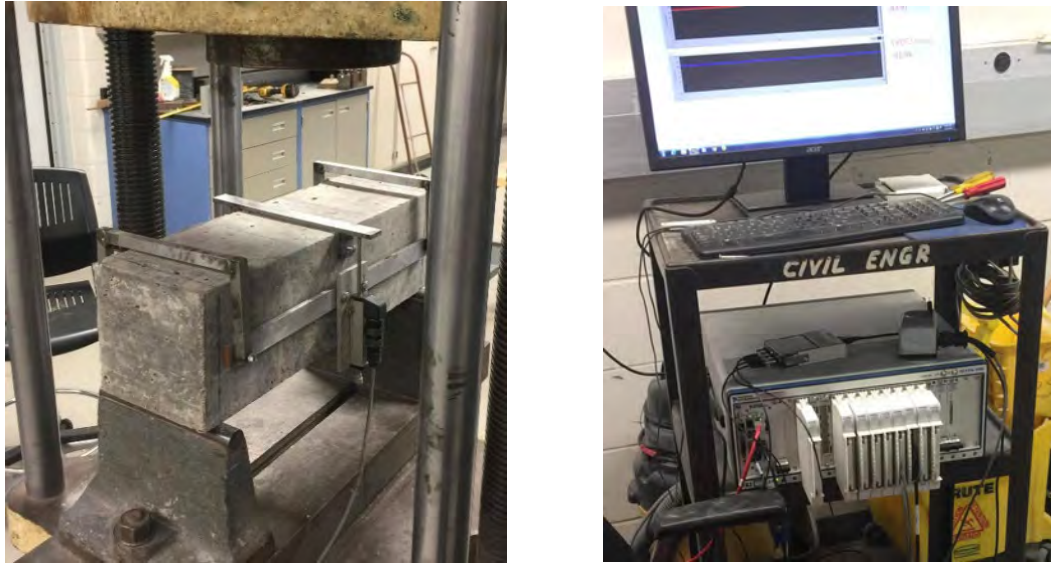
Figure 3.15 Specimen test setup and data logger.
