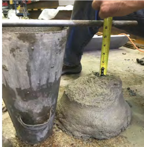
Figure 6.5 Slump test for non-FRC slab
