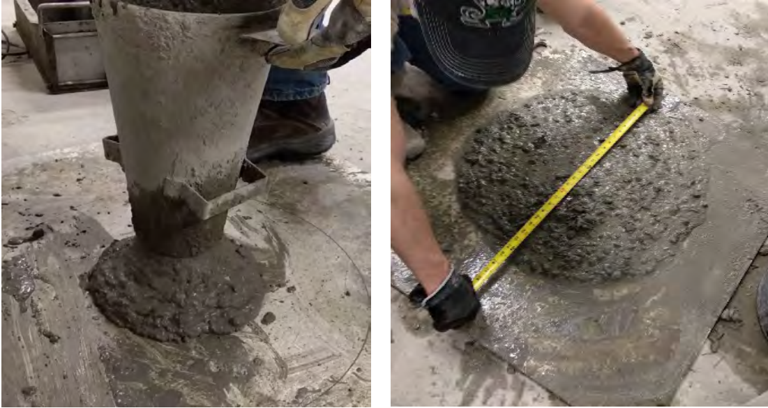
Figure 5.2 Slump flow test
