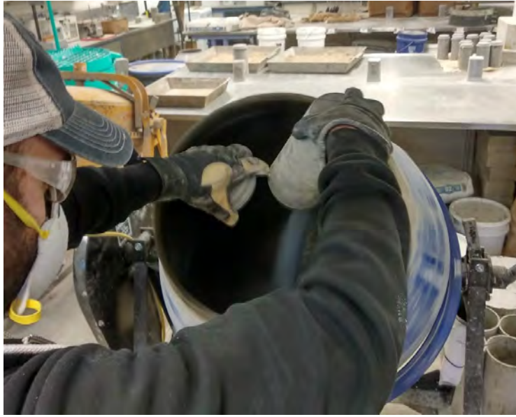
Figure 5.1 Loading silica fume
