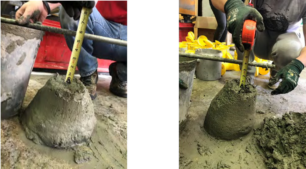
Figure 6.10 FRC slab slump test before and after fiber
