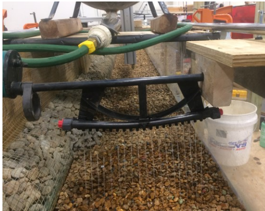
Figure 5.9. Continuous, uniform hot water seeding during IR data collection.
