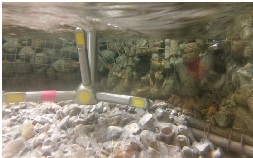
Figure 5.6. Side-looking SonTek ADV in flume.
