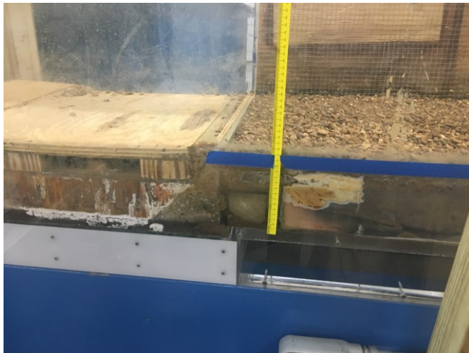
Figure 3.7. Outlet step at the end of the flume test section.
