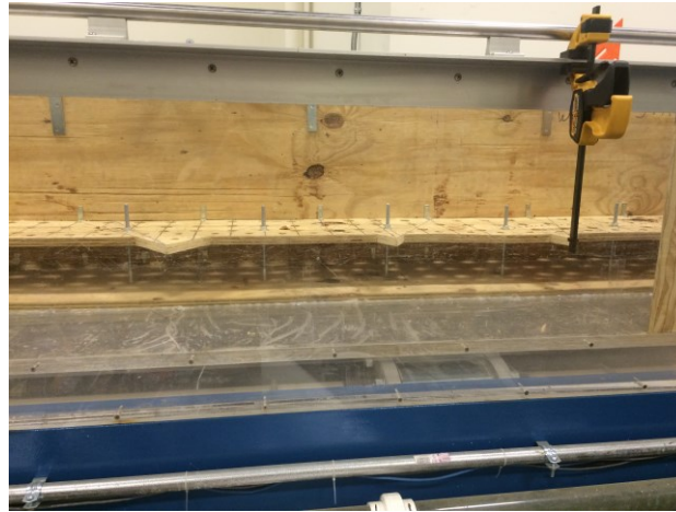
Figure 3.11. Platform constructed in ELJ test section and installed in the flume.
