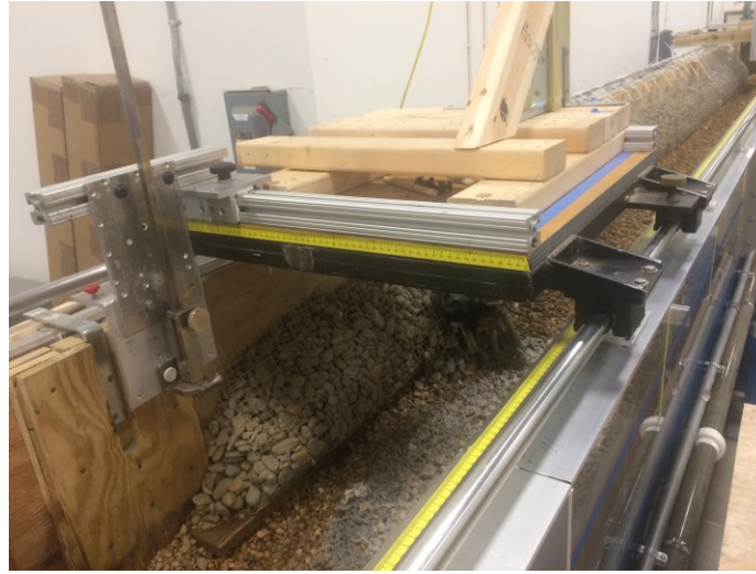
Figure 3.9. Movable trolley mounted to the flume rails and used for holding instrumentation.
