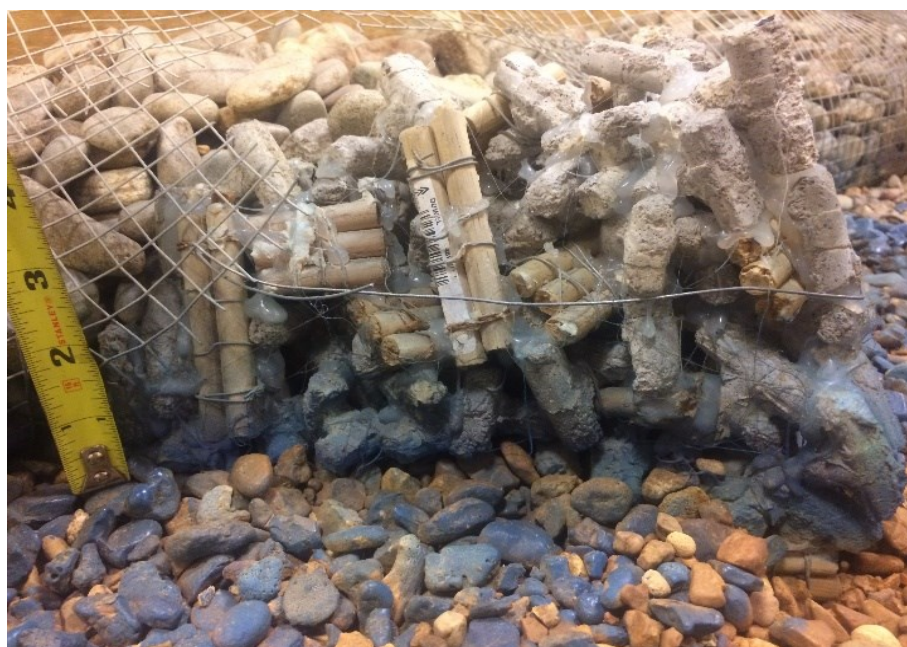
Figure 3.14. Oblique view of constructed ELJ3 model
