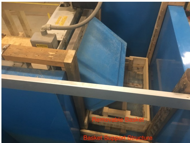
Figure 3.8. Sediment basket used to capture outgoing sediment from the flume outfall.
