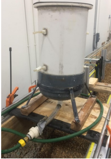
Figure 5.8. Reservoir for hot water supply during IR data collection.
