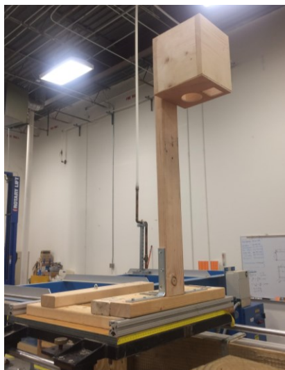
Figure 5.10. IR camera mount for plan-view data collection at ELJ3.
