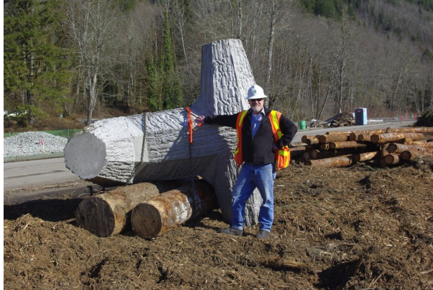
Figure 1.1. Standard concrete dolo, with textured surface recreating natural roughness. Human for scale. (WSDOT, 2011)
