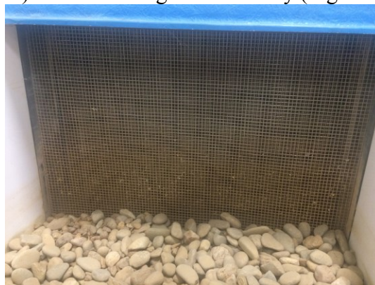
Figure 3.5. Flume inlet with rectangular grates and cobble bed entrance to promote uniform flow.
