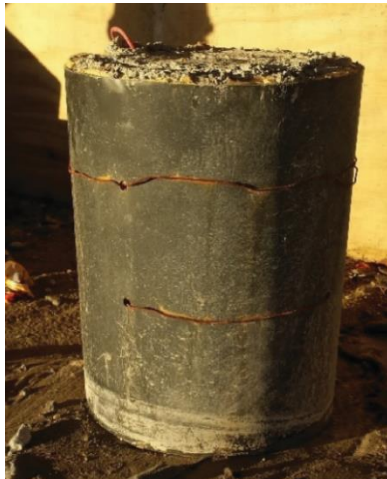
Figure 4.5. “Stress free” concrete cylinder.
