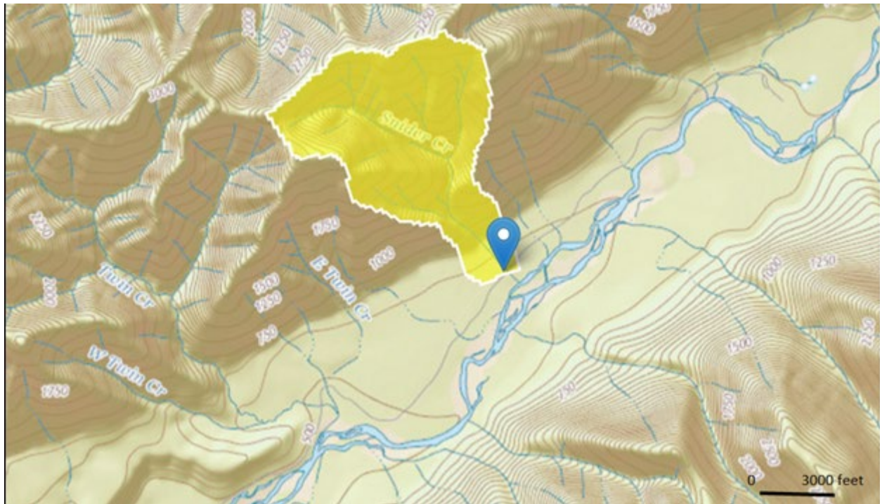
Figure 57. Snider Creek Culvert drainage area (USGS 2021).
