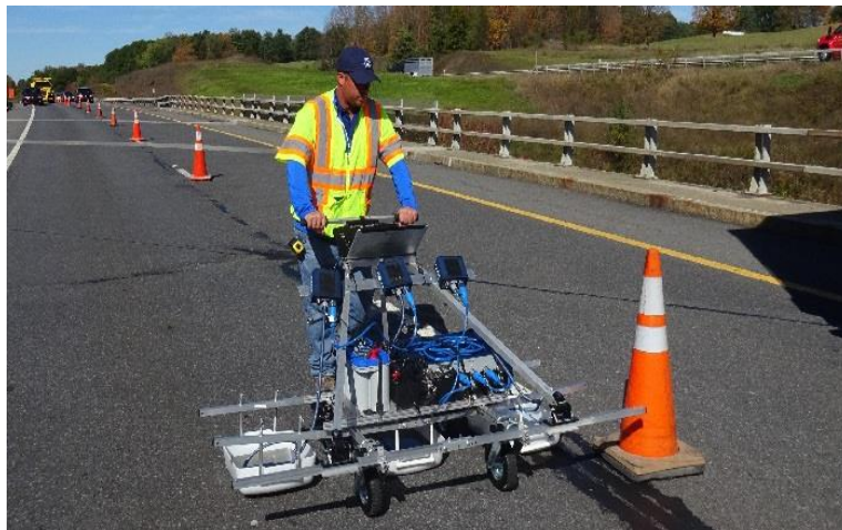
Figure 5. Ground Penetrating Radar Test.
