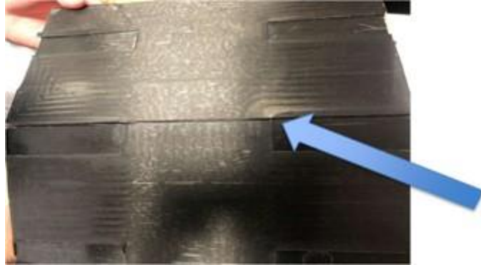
Figure 4. Damages along the thin regions of the cured carbon fiber plate.
