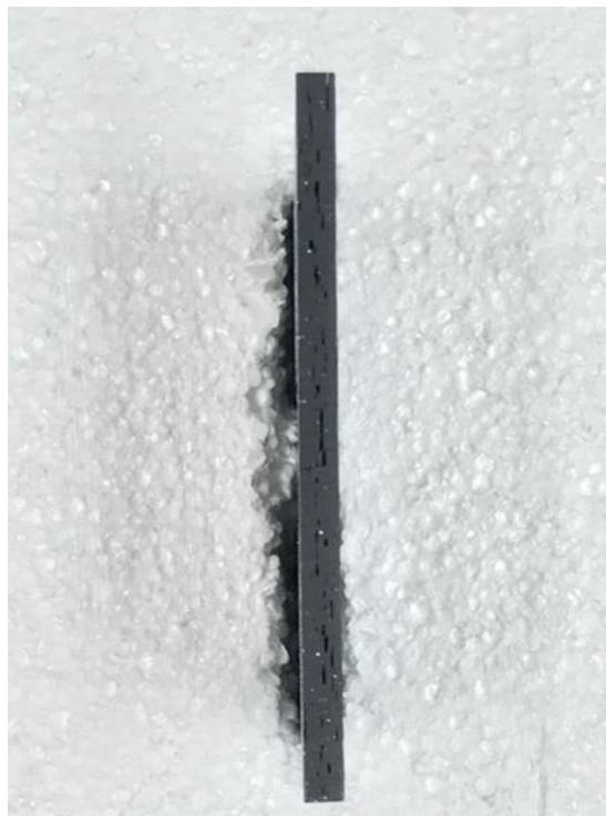
Figure 5. Delaminations on the SCC specimen.
