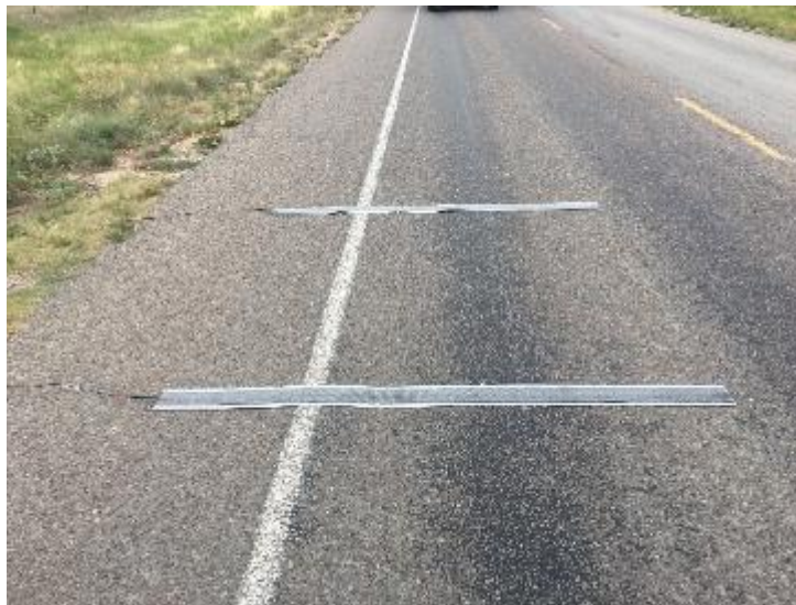
Figure 39. Imbedded Sensors on Top of Each Metal Plate.
