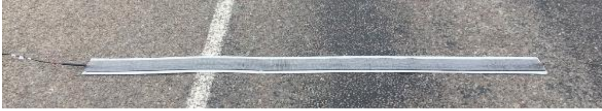
Figure 13. 4-Inch Pocket Tape with a Sensor Installed on the Road.
