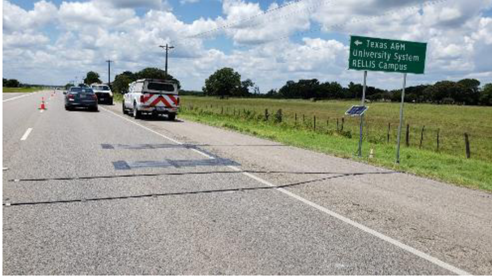
Figure 40. Portable WIM Demo-Monitoring Testing Station in SH 21 (WB), Bryan District.
