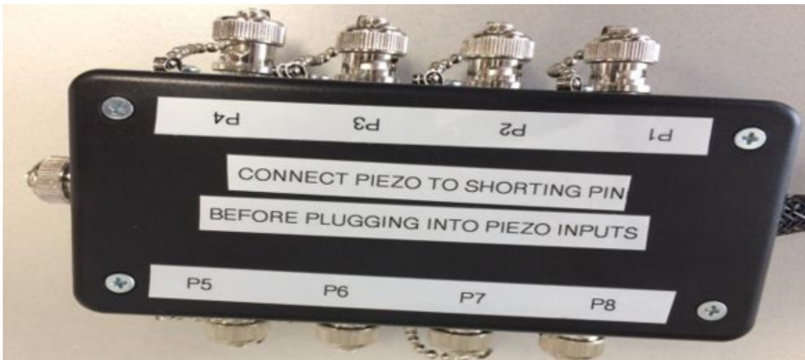
Figure I-2. TRS Piezo-electric Channel Connector with Eight Sensors Capacity, i.e., 4-Lane Setup.
