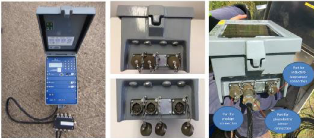
Figure I-1. Three-Channel TRS Portable WIM Unit. (Piezo-electric Channel (2 nd channel) = 8 Sensors or 4-Lanes).
