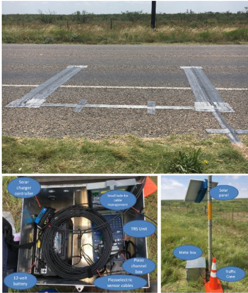
Figure I-4. Portable WIM System Main Components.
