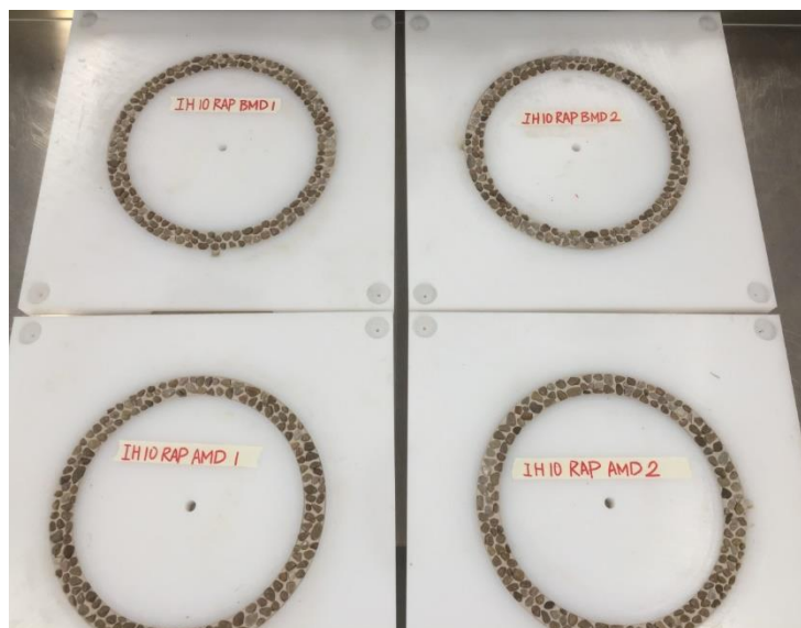
Figure 4-22. IH 10 RAP Aggregate Rings.
