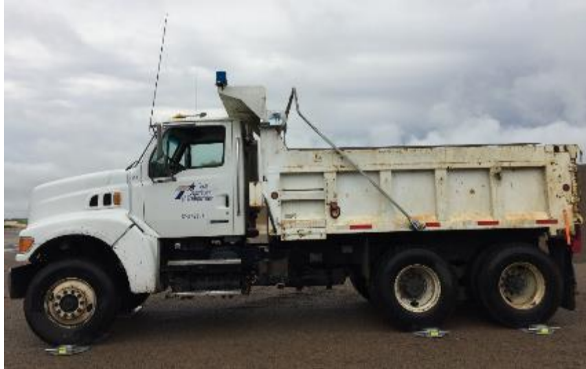
(a) Dump Truck Weighing Operation
