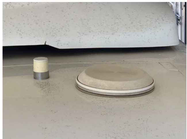
Figure 13. Radio Antennae Placement of Bus Roof.
