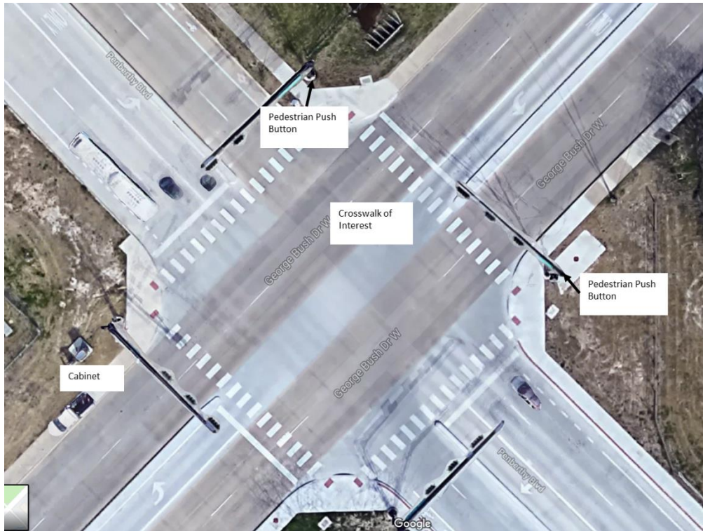
Figure 6. Pedestrian Push Button Locations at GBD/PB.
