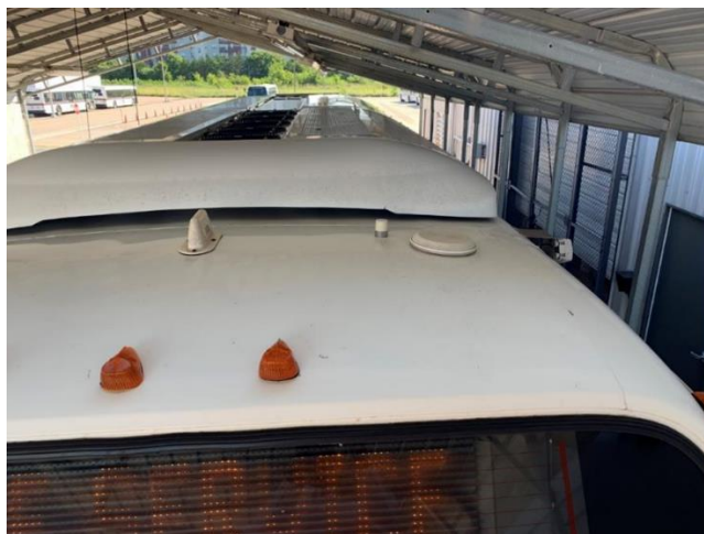
Figure 13. Radio Antennae Placement of Bus Roof.
