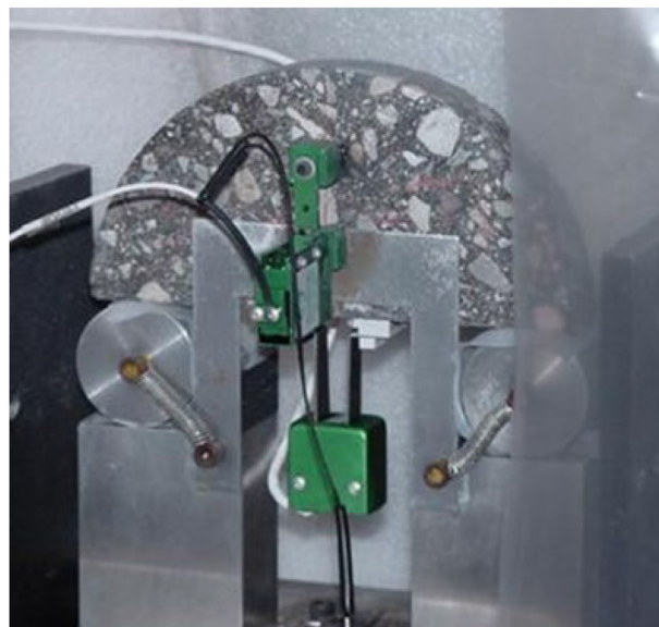
Figure A.2. Semi-Circular Bending (SCB) with a Crack Mouth Opening Displacement (CMOD) Test Setup (Marasteanu et al. 2012).
