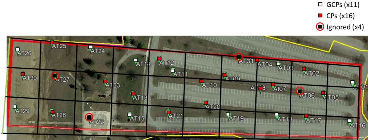
Figure 81: Positions of the Targets as GCPs for the 11 GCPs 3D point Cloud
