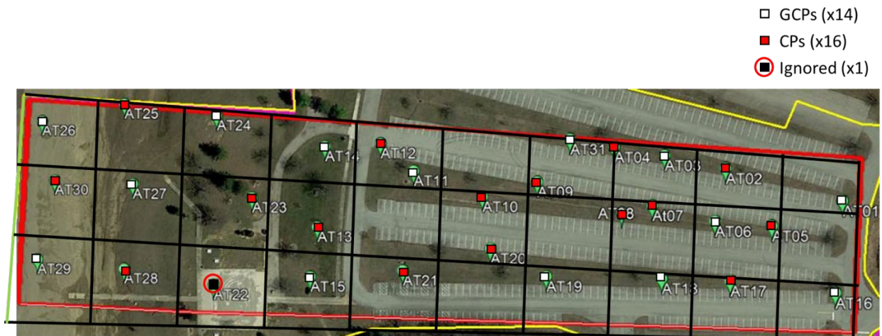
Figure 75: Actual Positions of the Vinyl Targets and Targets Selected as GCPs and Check Points
