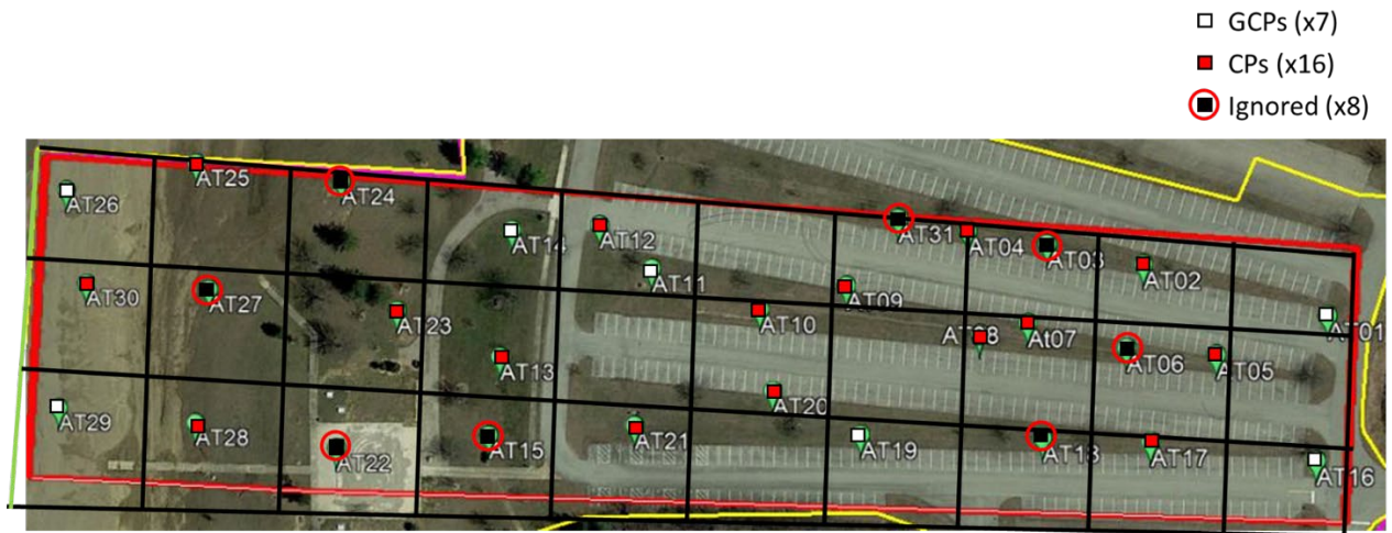
Figure 83: Positions of the Targets as GCPs for the 7 GCPs 3D point Cloud
