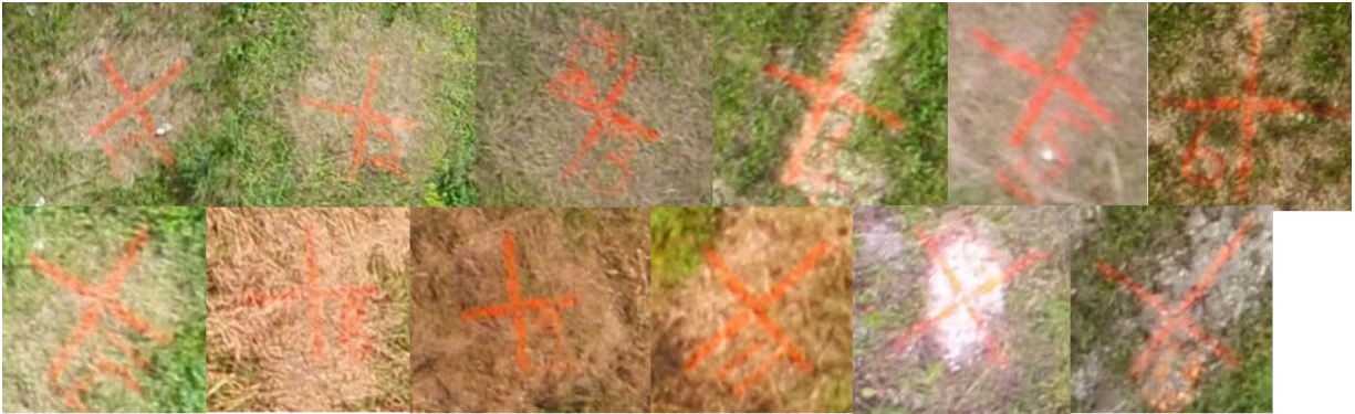
Figure 62: Images of the GCPs Marked on the Field for the I-75 Construction Site
