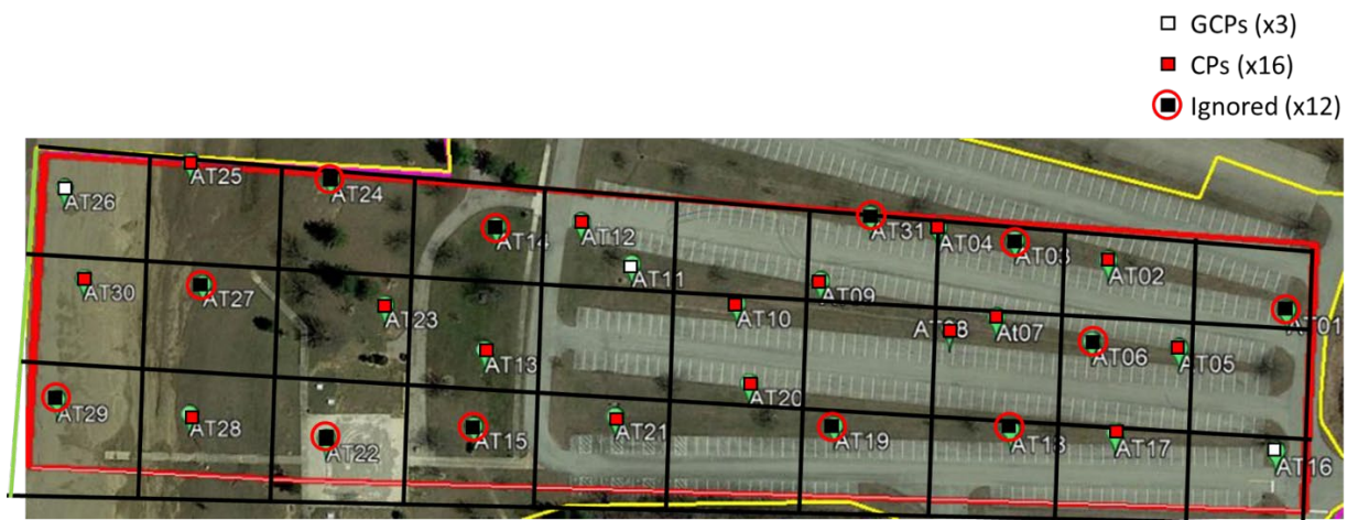
Figure 85: Positions of the Targets as GCPs for the 3 GCPs 3D point Cloud
