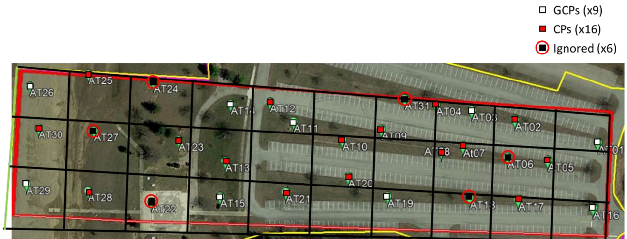
Figure 82: Positions of the Targets as GCPs for the 9 GCPs 3D point Cloud
