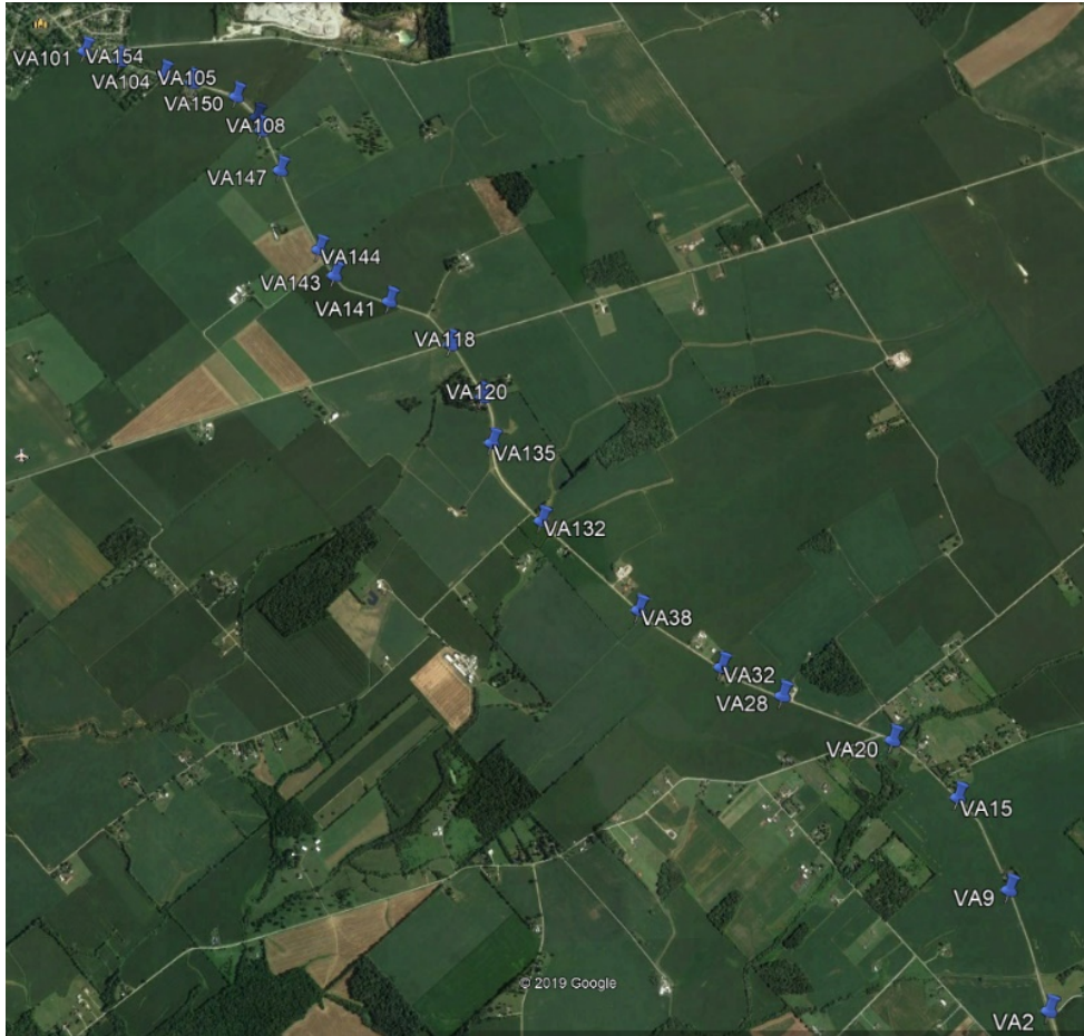
Figure 97: Location of the Good Mag-nails Used as GCPs to Process Version 2 of the Pix4D Project
