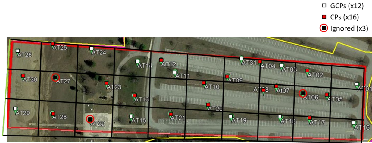
Figure 80: Positions of the Targets as GCPs for the 12 GCPs 3D point Cloud
