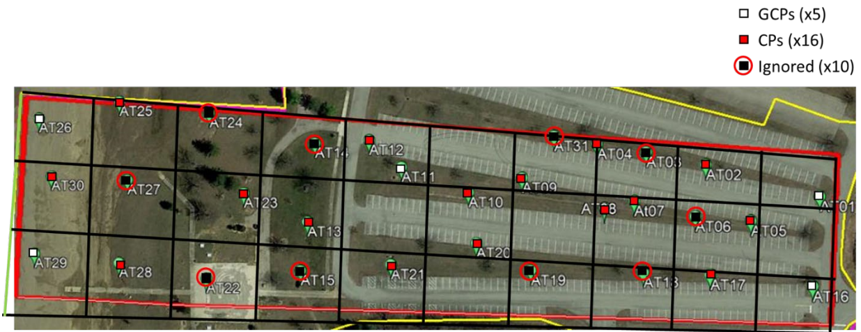
Figure 84: Positions of the Targets as GCPs for the 5 GCPs 3D point Cloud
