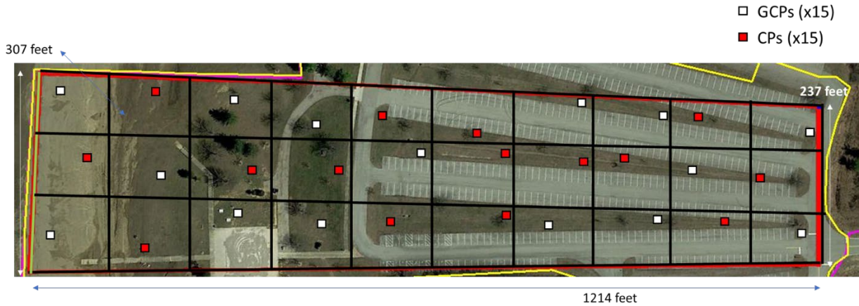
Figure 74: Map of the Region Mapped with Vinyl Targets Designated as GCPs and Check Points
