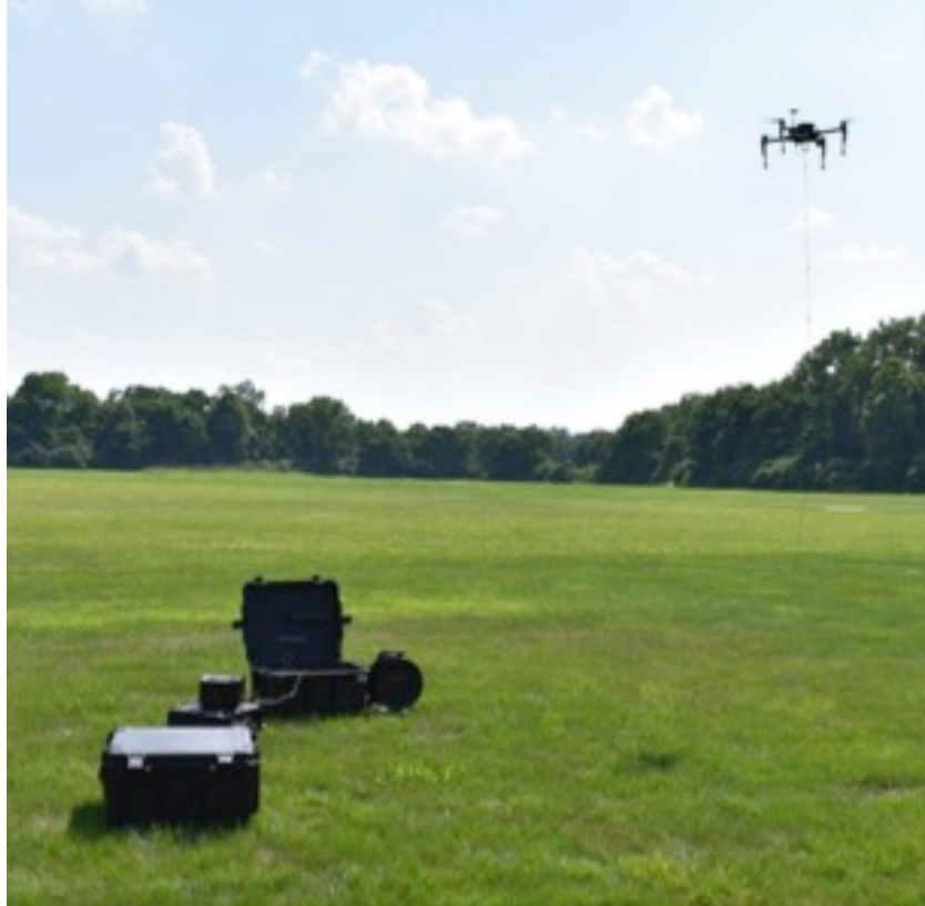
Figure 10: Powerline/M100 tethered platform
