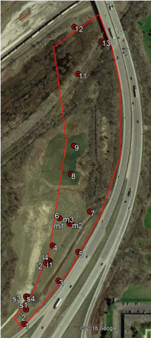
Figure 63: Locations of the GCPs Marked on the Region Mapped for the I-75 Construction Site
