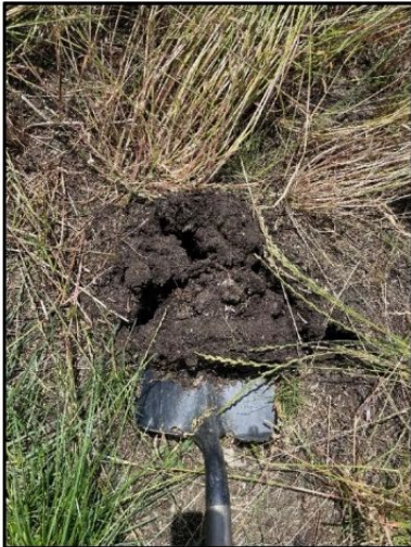
8SB4 Soil Revealed - mainly compost, little soil, very loose structure
