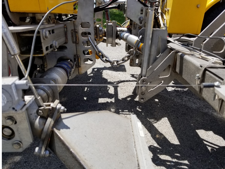
Figure 25 - TRC Inc. installed string potentiometer on the RT3 Curve device.
