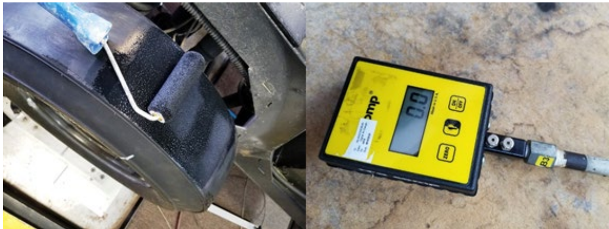
Figure 11 - Apparatus used for Contact Patch Testing of the ASTM E524 Tire.
