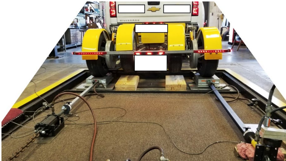
Figure 15 - Apparatus used for Force Plate Assessment of the RT3 Curve.
