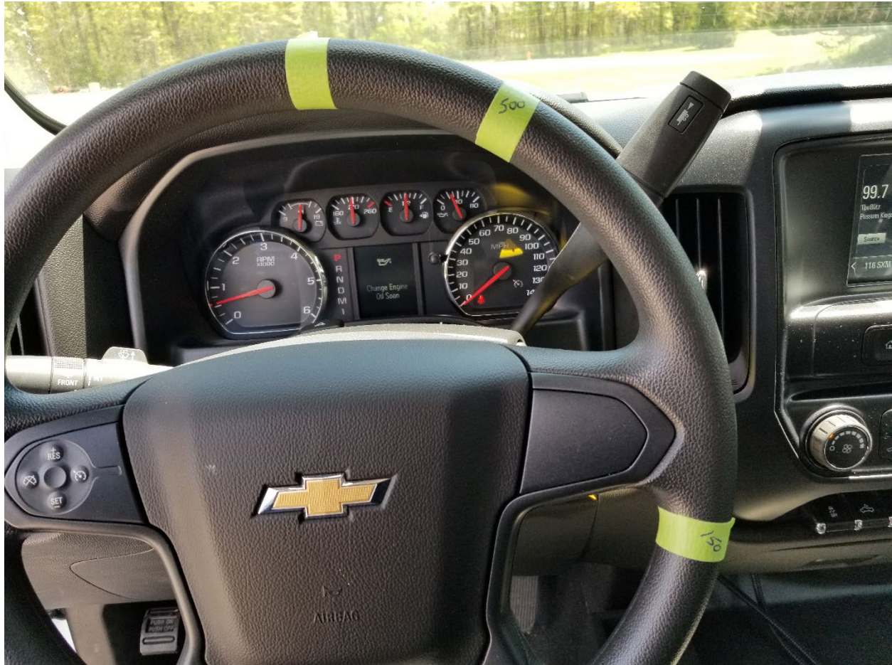
Figure 3 - Steering wheel of RT3 Curve truck taped with curve radius markers.
