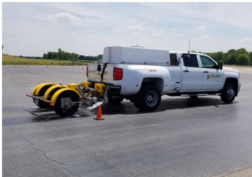
Figure 18 - RT3 Curve being tested on Jennite surface with instrumentation installed.
