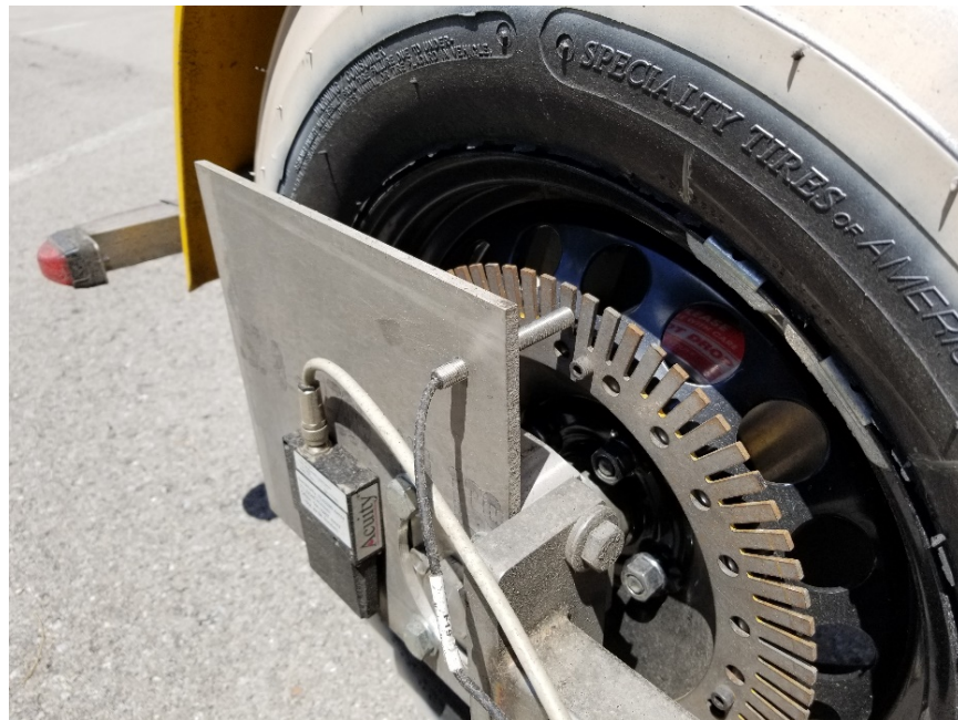
Figure 24 - TRC Inc. installed wheel speed and ride height sensors on RT3 Curve
