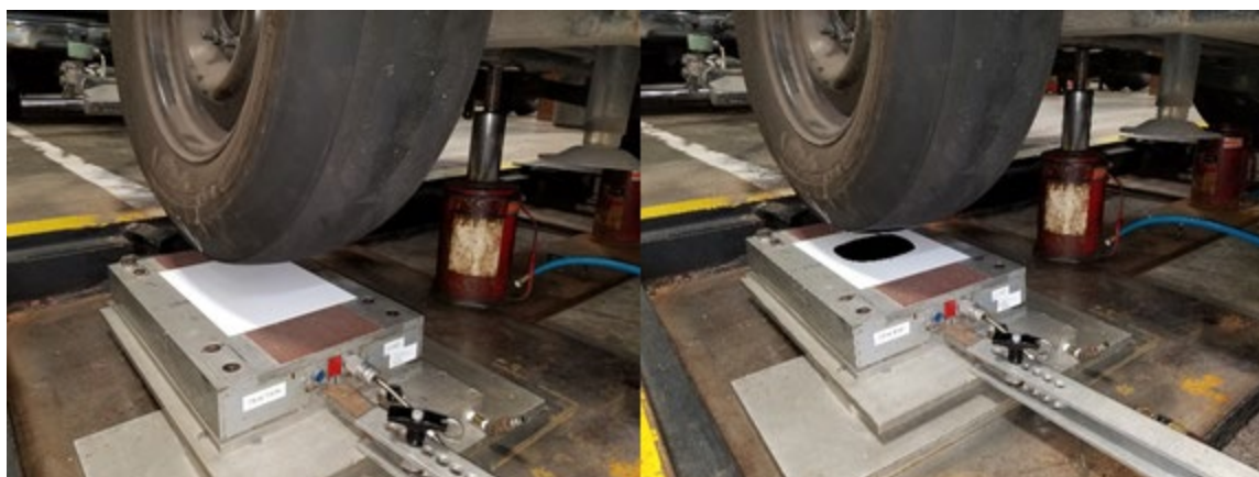
Figure 12 - ASTM E524 Tire over Force Plate A) No contact patch, B) With contact patch.
