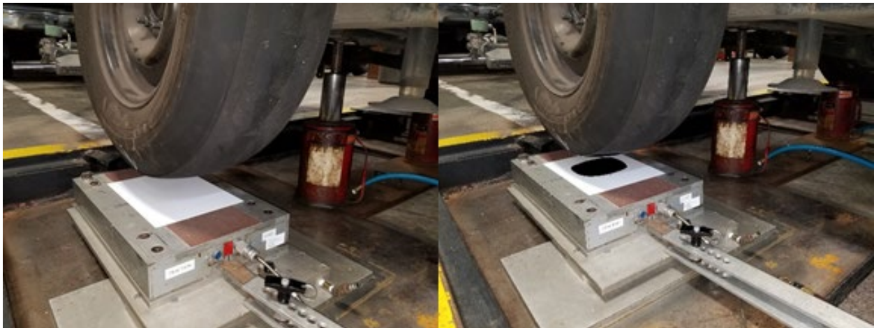
Figure 2 - Apparatus used for Contact Patch Assessment with the ASTM E524 Tire
