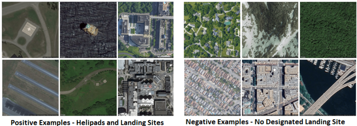
Figure 5: Sample aerial images from the dataset that we developed as a part of the project. While the term helipad is used for the positive set, the dataset also contains areas that helicopters are intended to land at, e.g., helicopter runways.
