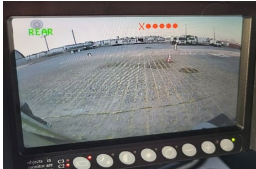
Fig. I-45: The Radar Detection is Matched with the Rear-view camera
