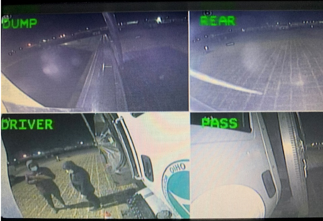
Fig. IV-3: Default Split-Screen View with Four Cameras
