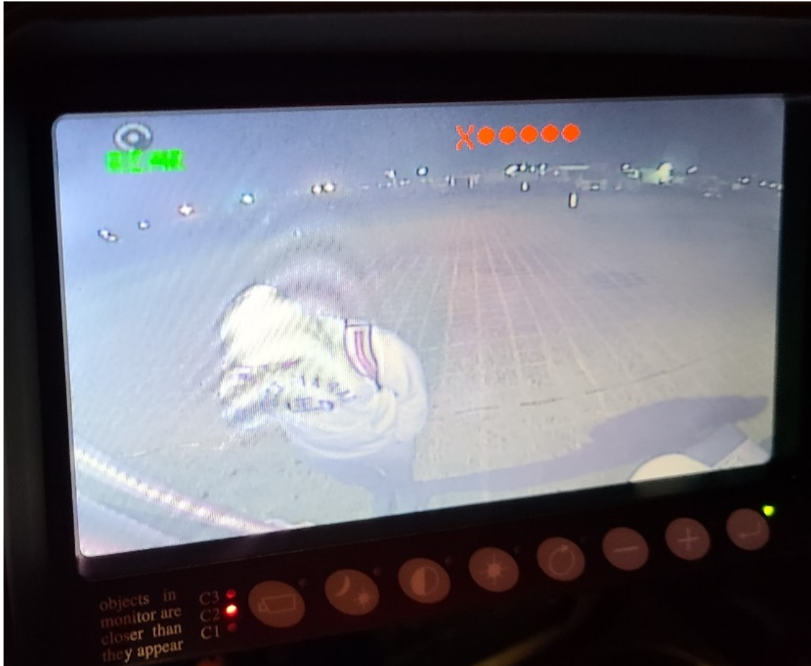
Fig. IV-6: Rear-view Camera and Radar Sensor Indicator on the Monitor When the Vehicle is in Reverse
