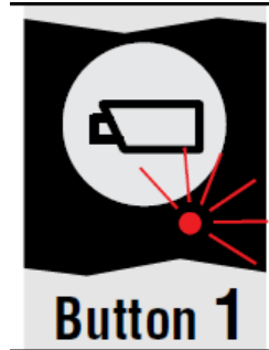
Fig. IV-4: Red LED under Button 1 indicating Manual Camera Selection Enabled.
