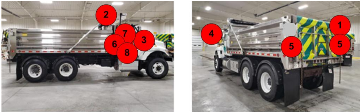
Fig. I-7: Installation Option using Strobe Light Cable Channels
