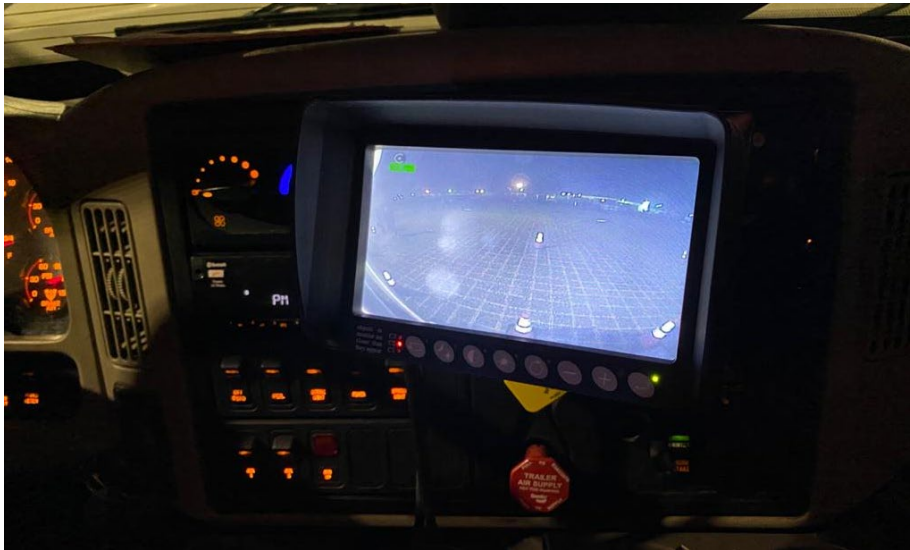
Fig. I-12: Dashboard Installation for Display
