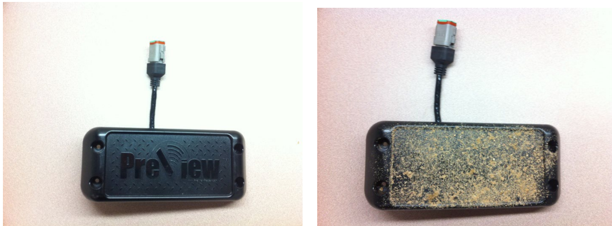
Fig. II-13: Normal and Soiled Radar Sensors (Fan et al., 2019)
