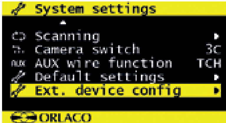
Fig. I-28A: System Settings Menu on the 12-inch Display
