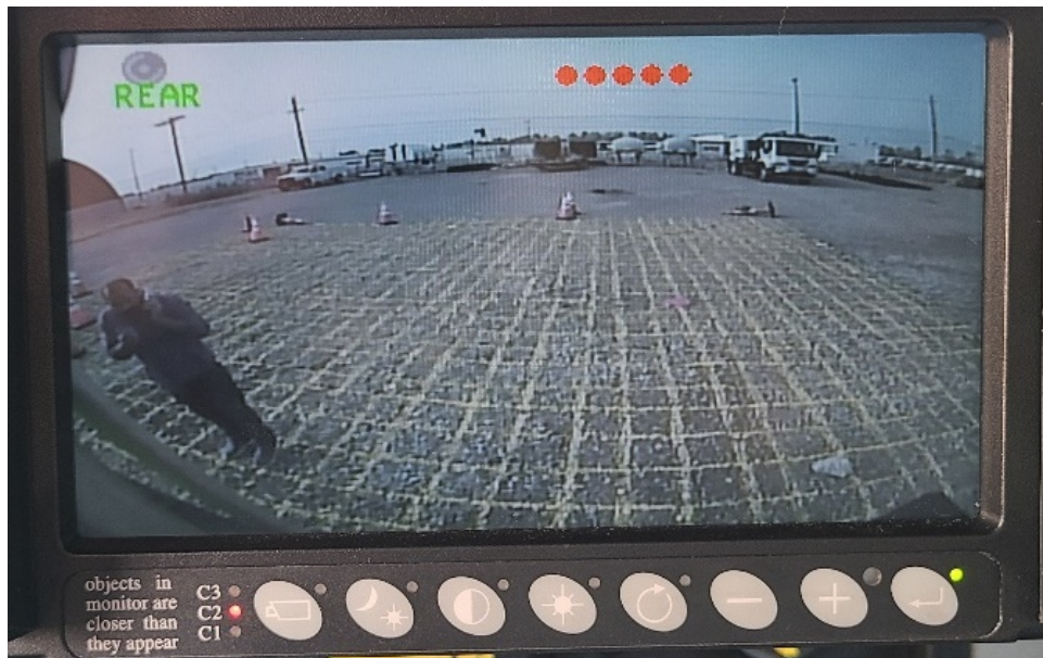
Fig. IV-7E: Five Red Dots Indicating Zone 5 (Closest to the Sensors)
