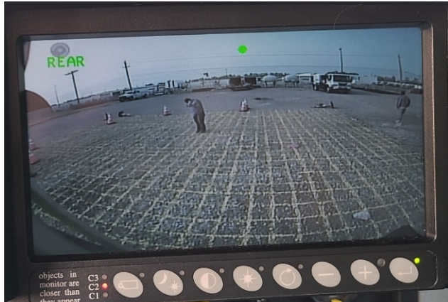
Fig. IV-7A: Single Green Dot Indicating Zone 1 (Furthest from the Sensor)
