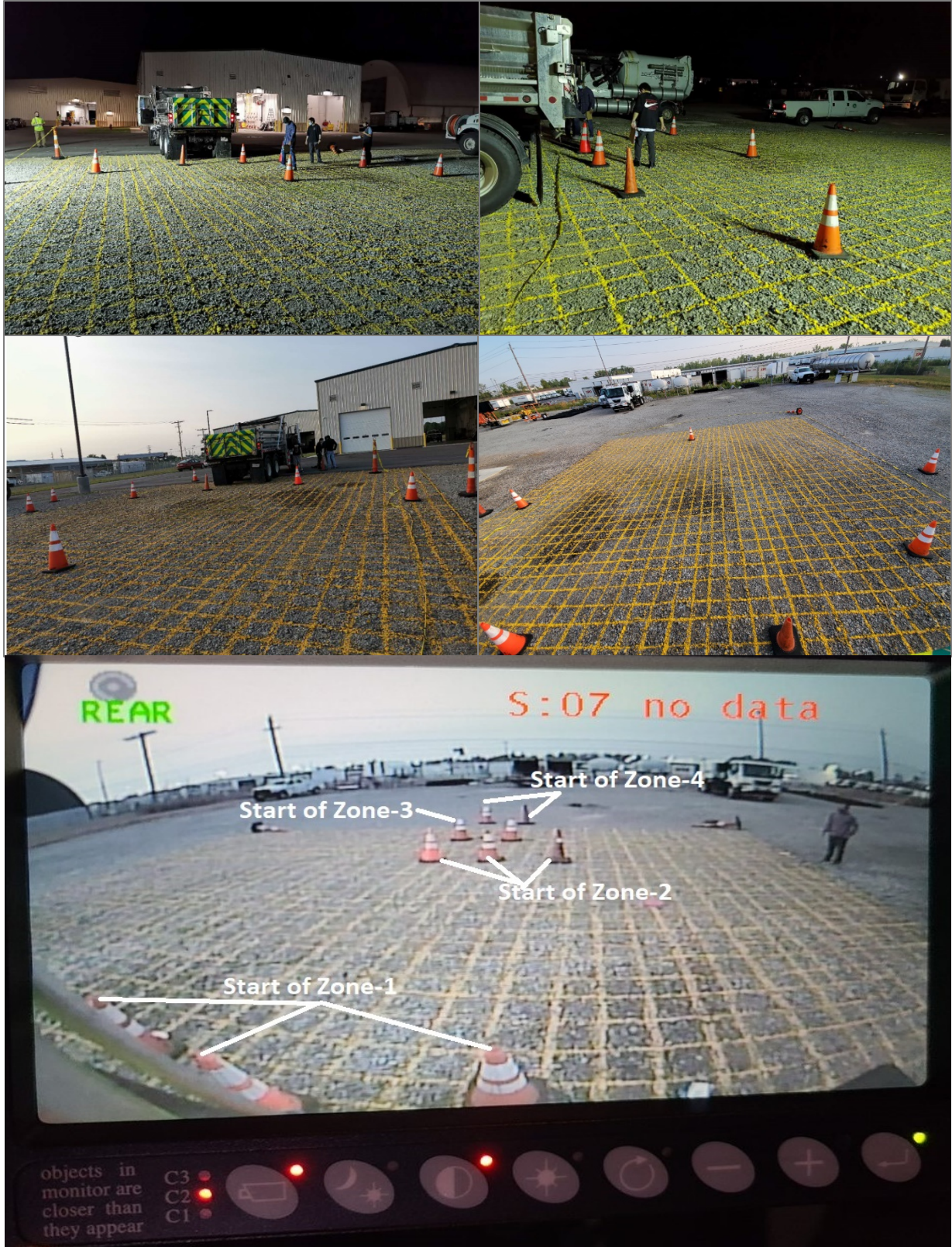
Fig. III-1: Testing Site with Layout of the Cones Measuring Camera Viewing Capability
