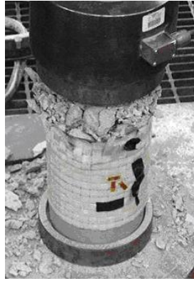
Figure 4-16. Sample CC3 after compression testing showing intact overlap
