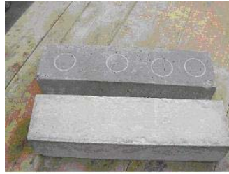
Figure 4-1. Two 3"x4"x16" prism samples, one sandblasted and prepared for pull-off testing
