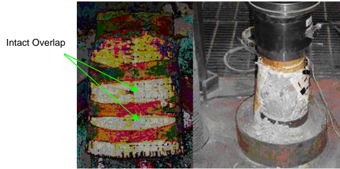
Figure 4-11. Sample CC1 after compression testing showing intact overlap
