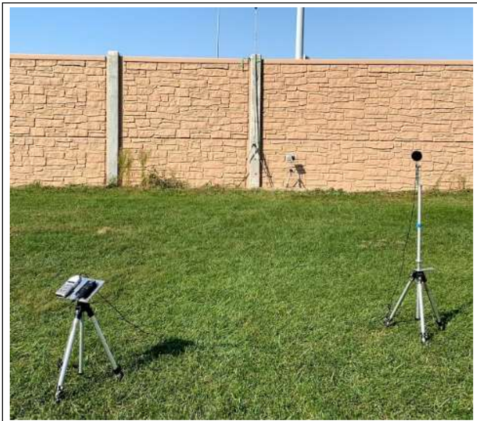
Figure 4: Typical Setup for Traffic Noise Measurement Equipment
