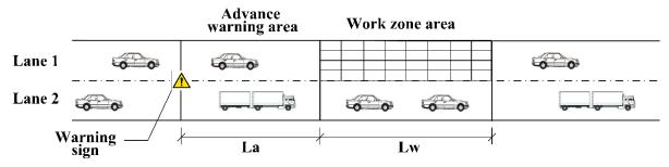
Figure 2.2 Configuration of a typical work zone
